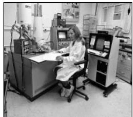
Scientist using a scanning electron microscope to study the mineralogy of a meteorite.
