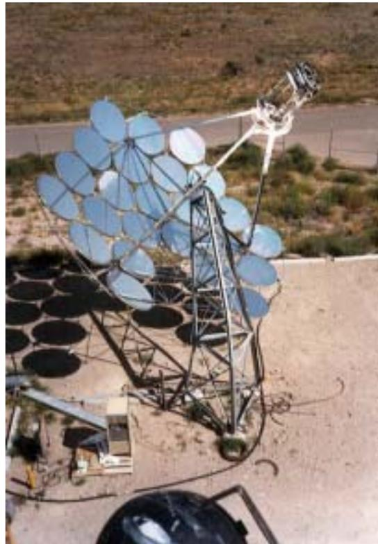
**Figure 15. A 5-kilowatt point-focus Stirling engine concentrator system. (Cummins Power Generation, Inc./PIX01730)**
