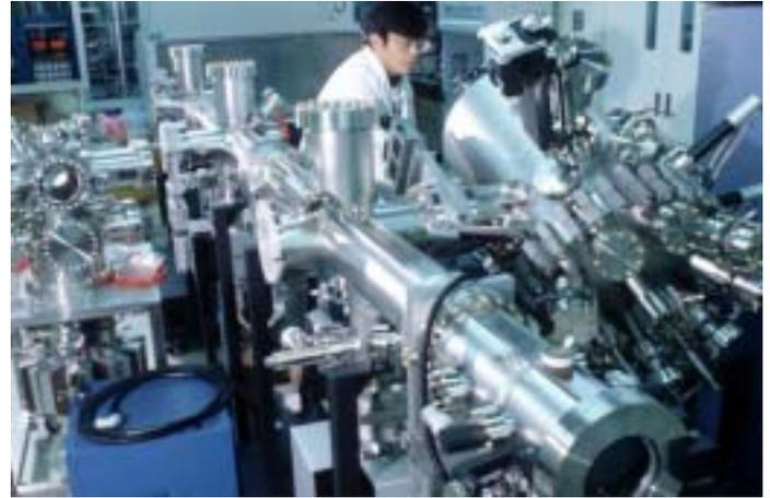
**Figure 21. Molecular-beam epitaxy system. (Warren Gretz/PIX01144)**
