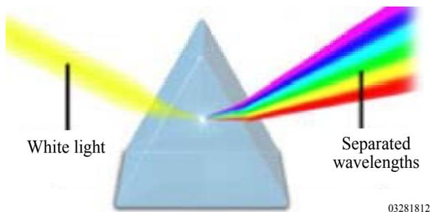
**Figure 12. Refraction of light through a prism.**
