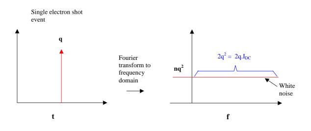
in<sup>2</sup> =  $2nq^{2}\Delta f = 2qI_{DC}\Delta f$   $I_{DC} = bias current; q = electron charge$
