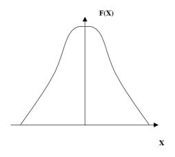
As noise is random then it's mean value will be zero, hence we use **mean square** values, which are measurements of the dissipated noise power. The effective noise power of a source is measured in **root mean square** of **rms** values.
