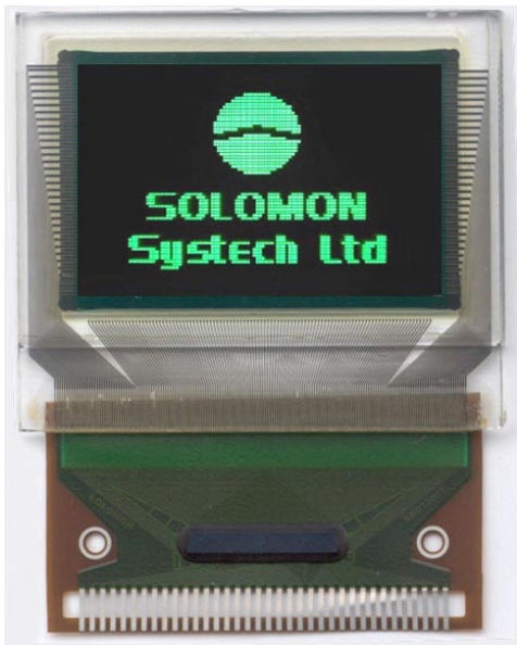
Fig. 3 Solomon Systech OLED Driver IC SSD1301T
