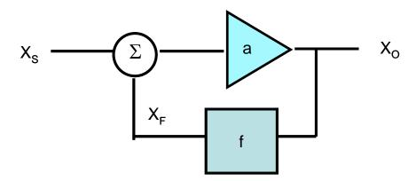
A feedback amplifier: with positive feedback. Gain with feedback is
