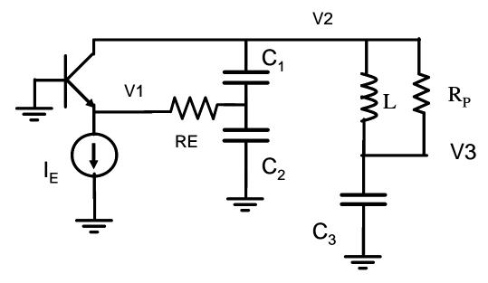
The resonator is modified by adding a capacitor C3 in series with the inductor L. Since this branch of the circuit should remain inductive, L must be increased from its Colpitts value.
