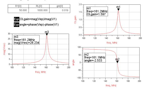
Note that the peak OL gain simulated is less than the analysis predicted; 1.6 vs. 3. Replacing the device with a Voltage controlled Current source (VCCS), the simulations
