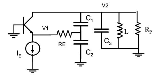
RE can help reduce the phase shift by making  $-re+RE>>\omega C_2$
