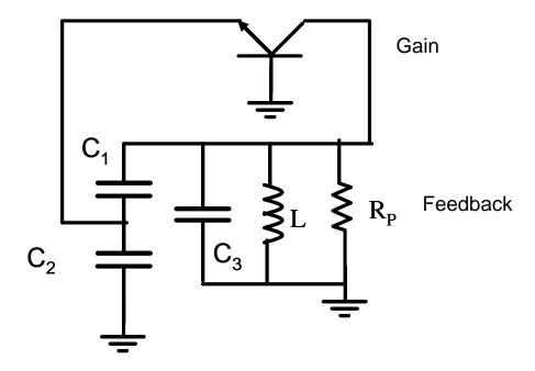
In this configuration the active device is in a common base configuration. The open loop gain will be set by the gm of the device, by Rp and the capacitive divider. The frequency of oscillation is determined by the resonator as in the previous examples.
