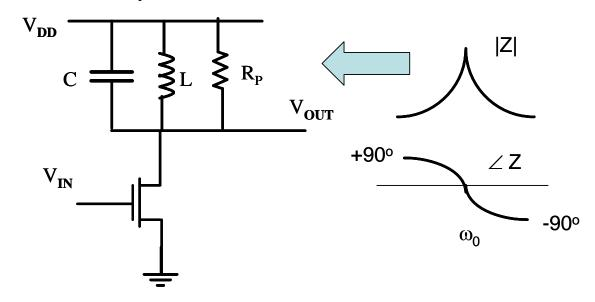
Load: The impedance of the resonator peaks (= Rp)and the phase is  $0^{\circ}$  at  $\omega_0$ . The susceptances of the L and C cancel at resonance.
