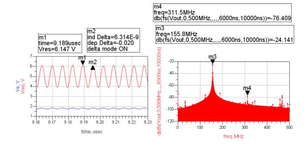
We see that the oscillator has reached a limiting amplitude of 1.147V. Note that the oscillator is current limiting, not voltage limiting because  $V_{CB} = Vres - Ve$  never drops below 2V. The resonator amplitude seems to be predicted by  $Vres = I_C*(RP||N^2/gm)$ , off
