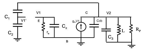
We also need to consider the effects of the device capacitors on the frequency.
