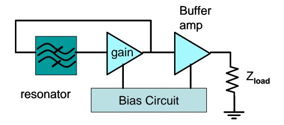
For oscillation to begin, open loop gain  $A\beta \ge 1$  and  $\angle A\beta = 0$ .
