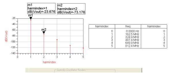
The spectral output from HB for the example oscillator is shown above. Harmindex represents the harmonic frequency.
