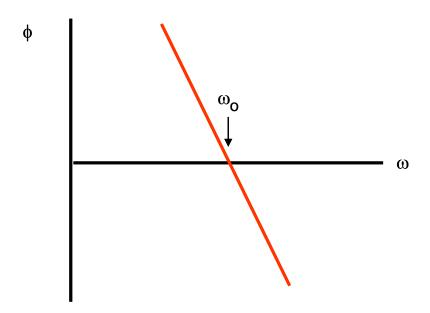
You can see that a change in phase  $d\phi$  will result in a change in frequency  $d\omega$ .
