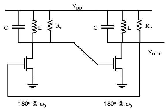
If  $(g_m R_P)^2 \ge 1$ , this circuit will oscillate. It can only oscillate at  $\omega_0$ , because only at that frequency will we have a total phase shift of  $0^\circ$ .
