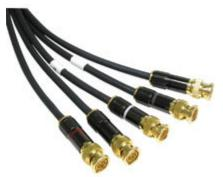
A five-wire format using 75-ohm coaxial cable (often in the form of a "snake"), RGBHV sends the three primary color components on three of the conductors and sends a horizontal and a vertical negative TTL (transistor-to-transistor logic) sync signal on the remaining two conductors – hence the Red, Green, Blue, Horizontal and Vertical which make up the RGBHV moniker.
