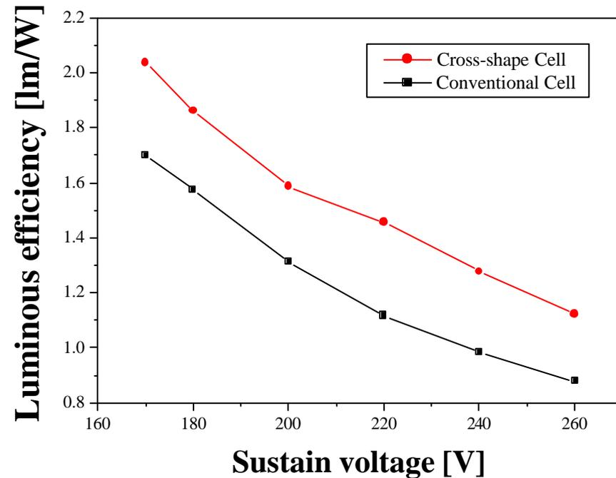
The luminous efficiency of the cross-shape cell with a high Xe percent (10%) is shown to be **2.0 lm/W** at the sustain voltage of **170 V**
