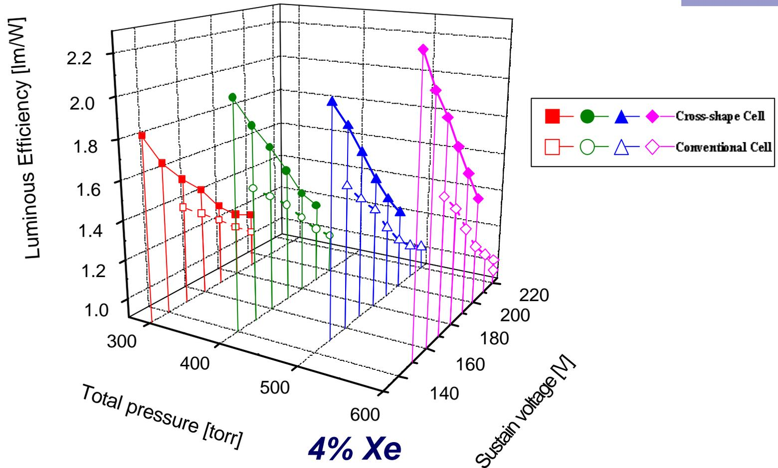
Compared with the conventional structure, the **cross-shaped cell structure** shows the **higher pressure**, the **higher luminous efficiency**
