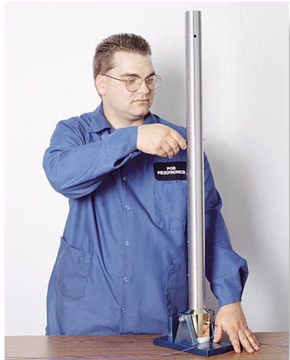
Test engineer calibrates sensor using 913B02 Hydraulic Impulse Calibrator with tourmaline reference standard.
