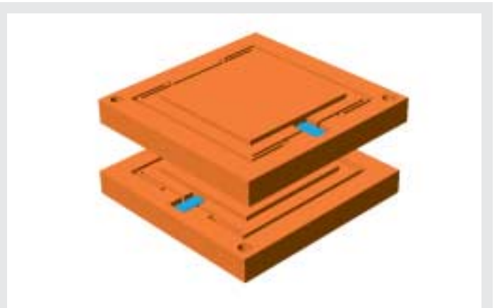
Fig. 50 a. Working principle of a stacked XY piezo stage (serial kinematics). Advantages: Modular, simple design. Disadvantages compared with parallel kinematics: More inertia, higher center of gravity, moving cables (can cause friction and hysteresis). Integrated parallel metrology and active trajectory control (automatic off-axis error correction) are not possible.
