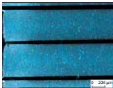
Piezoceramic layers in a "classical" stack actuator (HVPZT).
