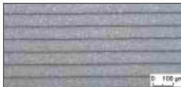
Piezoceramic layers in a monolithic actuator (LVPZT).
