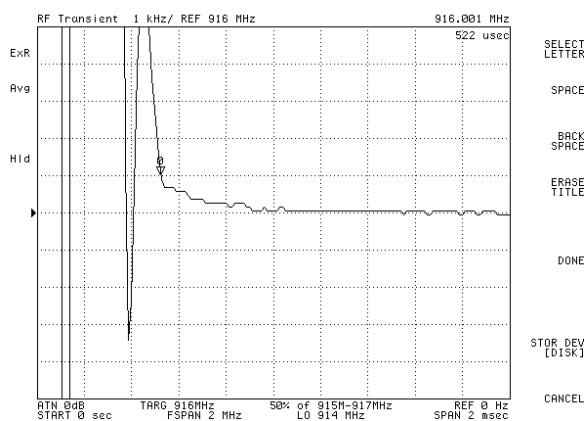
RF PLL Lock Up Time = 522μs (890 MHz → 916 MHz, within ± 1kHz)
