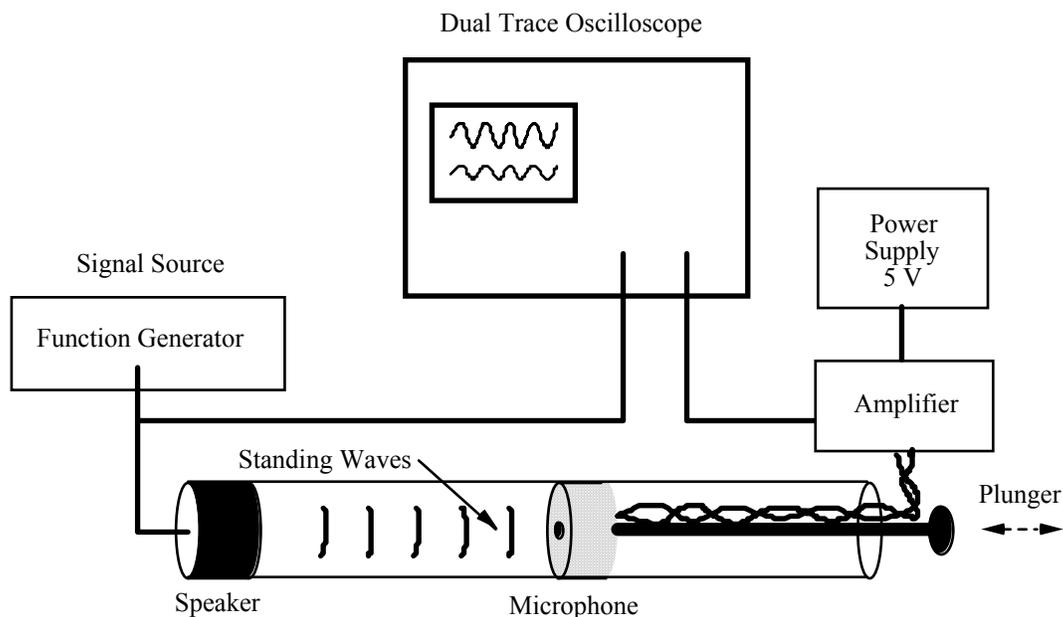
The waves in this setup are made by a small loudspeaker attached to a sine wave (function) generator. The speaker sets the air molecules into longitudinal vibration (vibration in the direction of wave propagation). The speaker always acts as a displacement antinode because the surface of the vibrating diaphragm sets the air molecules into motion. Set the generator at a frequency near 1000 Hz. The sine-wave generator should not be set at the maximum-amplitude or the loudspeaker will be damaged.
