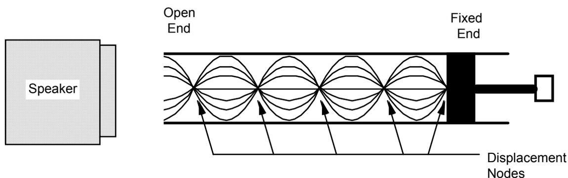
The reason for this condition is easily seen. A displacement antinode forms at the open end of the tube. Displacement is the range of the vibrating air molecules, and an antinode is where it oscillates as a maximum. At the closed end the displacement variations are very small as the waves compress the air molecules and are reflected at the surface of the
