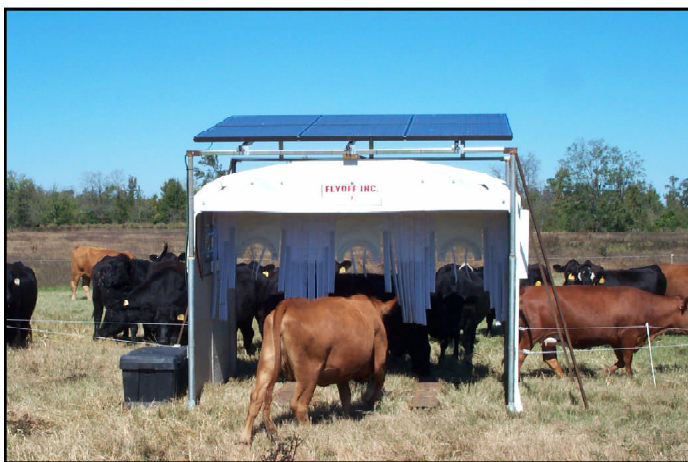
Figure 4: PV powered fly zapper at the Center for Environmental Farming Systems in Goldsboro, NC.
