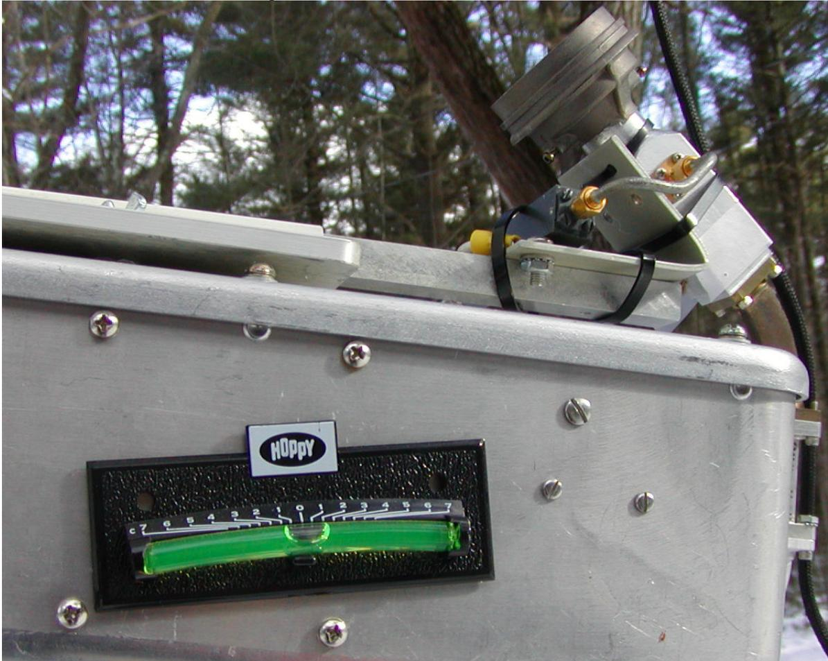
**Figure 16 - RV Level Indicator shows Dish Tilt**
