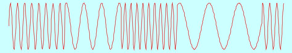
also used in Frequency-shift keying - where mark/space ratio changes, not f
