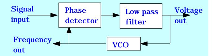
phase comparison with VCO generates error voltage...
