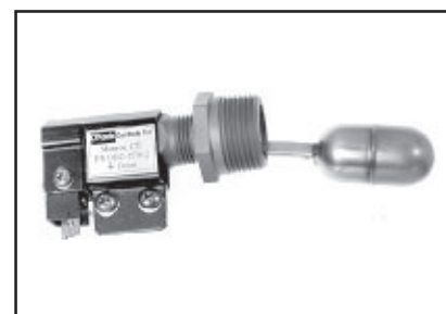
Horizontal float valve for side mounting to vessel. Float operates air valve on outside of vessel. Normally closed or normally open.
