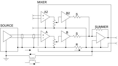
The pin 1 problem can be identified by a simple test, requiring only a device to inject current into a ground pin, as shown above. A low voltage transformer is coupled with a current limiting resistor to drive approximately 100 mA into a short circuit. A diode is added to chop the waveform in half, giving it plenty of upper harmonics for audibility.
