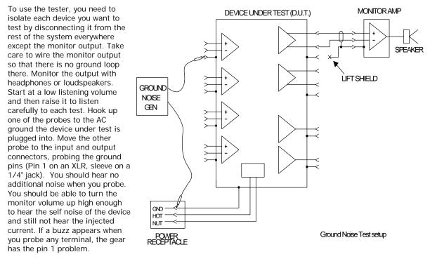
If you find a piece of equipment with a pin 1 problem, you might consider modifying it by re-routing the shield terminals directly to the chassis internally. Take care though -- you may be voiding a warranty by doing this!
