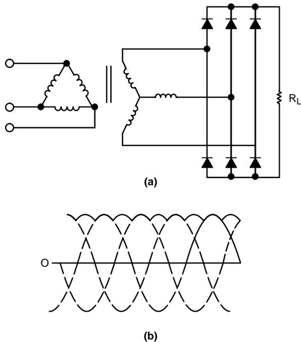
**Figure 95. Three-Phases Full Bridge Circuit and Associated Waveforms.**
