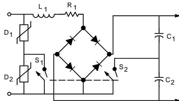
Figure 142. MOV Protection for a Universal Input Rectifier
