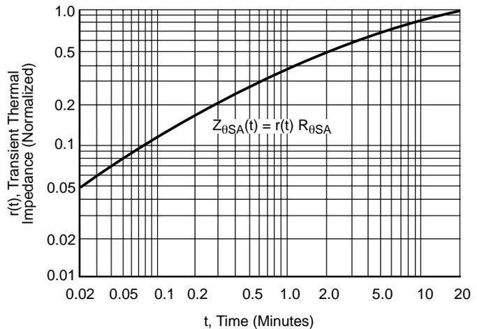
Figure 210. Thermal Response of Typical Category 1 Heatsink
