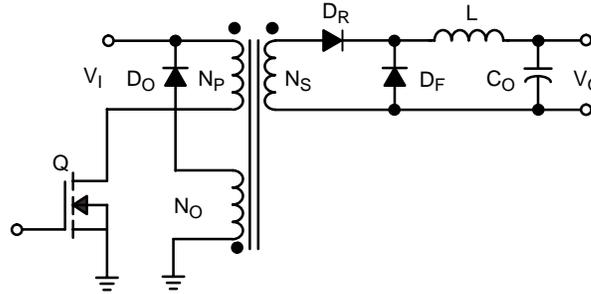
Figure 160. Output Section of a Forward Converter
