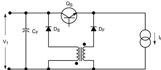
Figure 181. Buck Converter with "Lossless" Turn-on Snubber
