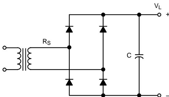
Figure 115. Bridge Circuit Used for Example Design
