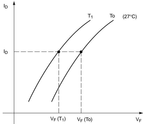
**Figure 62. Typical Forward-bias Diode Voltage Temperature Characteristics**
