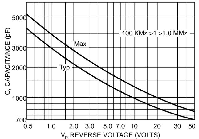
**Figure 22. Capacitance Versus Reverse Voltage For Schottky Rectifier**
