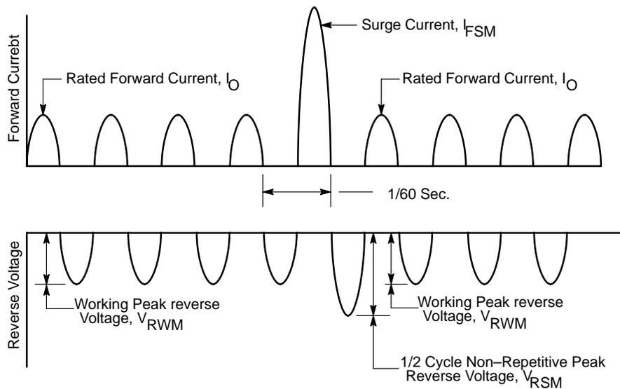
Figure 79. Conditions for the JEDEC Surge Current Specification
