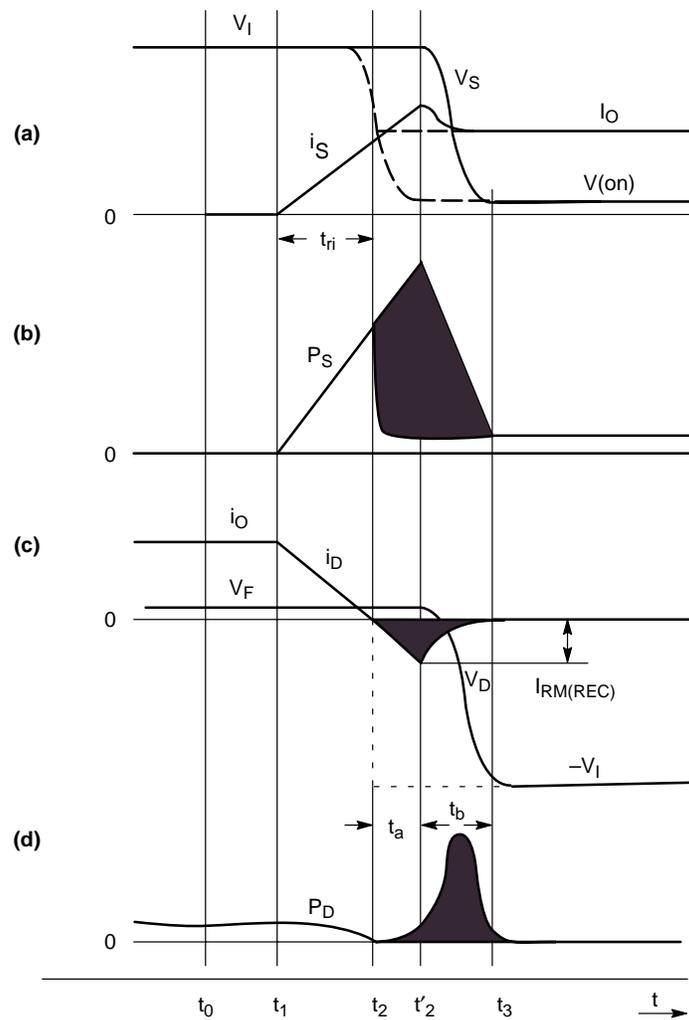
**Figure 162. Forced Commutation Waveforms: (a) Power Switch Voltage and Current; (b) Power Switch Dissipation; (c) Diode Voltage and Current; (d) Diode Dissipation. Diode Forward Drop and Switch On-State Levels Are Exaggerated**
