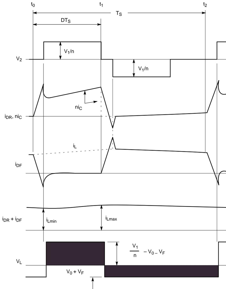
Figure 188. Forward Converter Waveforms for Continuous Mode Operation
