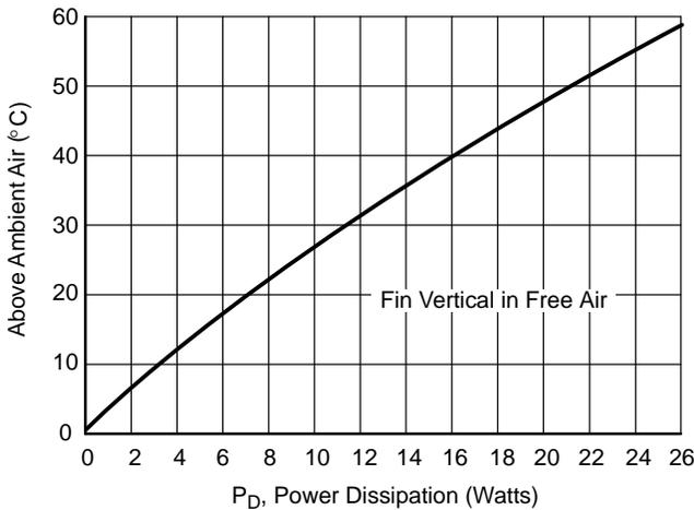
Figure 209. Typical Category 1 Heatsink Natural Correction Thermal Characteristics
