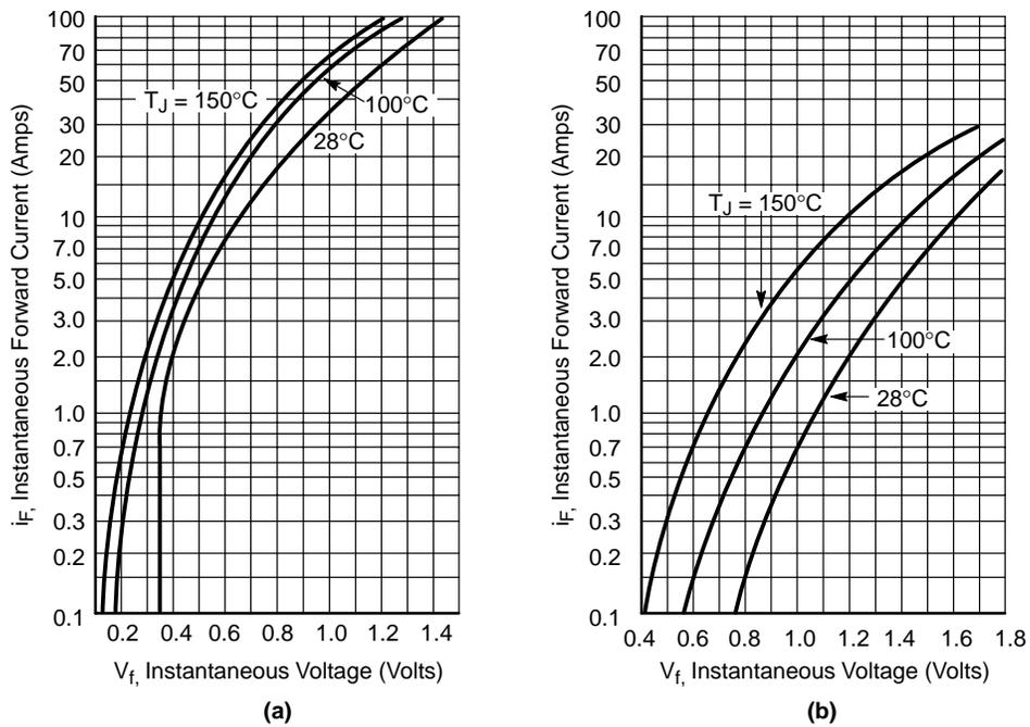
Figure 20. Typical Forward Voltage Characteristic
