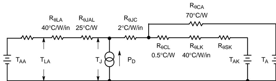
Use of the above model permits calculation of average junction temperature for any mounting situation. Lowest values of thermal resistance will occur when the cathode lead is brought as close as possible to a heat dissipator, as heat conduction through the anode lead is small. Terms in the model are defined as follows:
