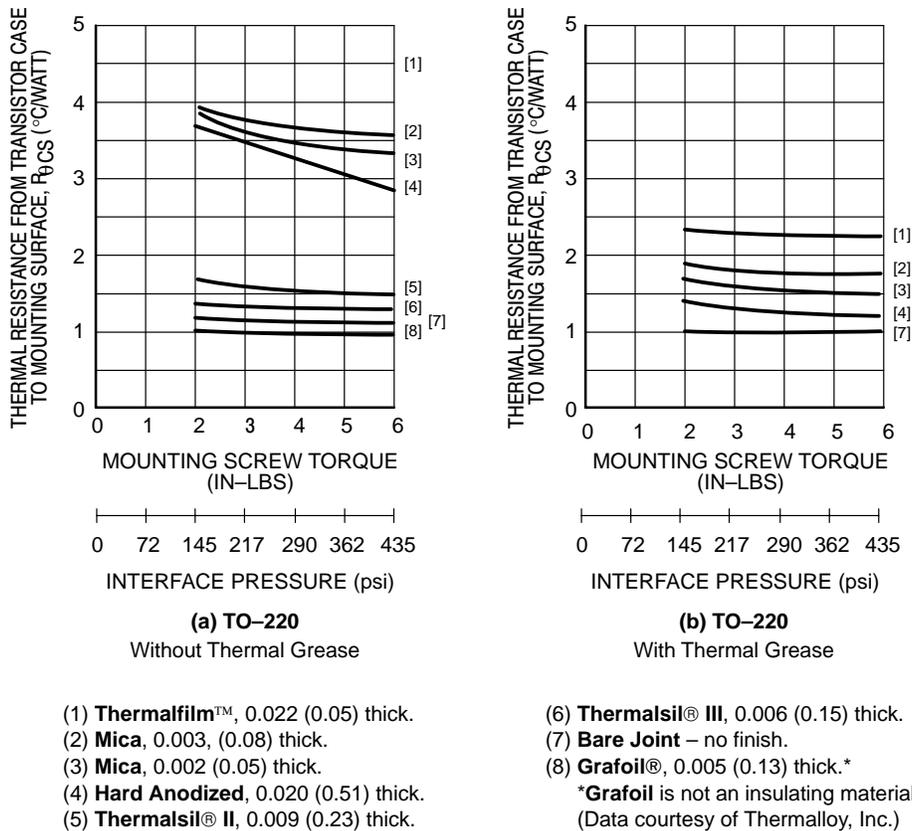
Figure 225. Interface Thermal Resistance for a TO-220 Package
