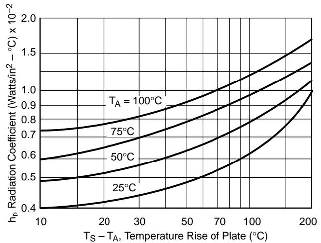
**Figure 203. Radiation Coefficient for a Black Body having an Unobstructed Pattern**
