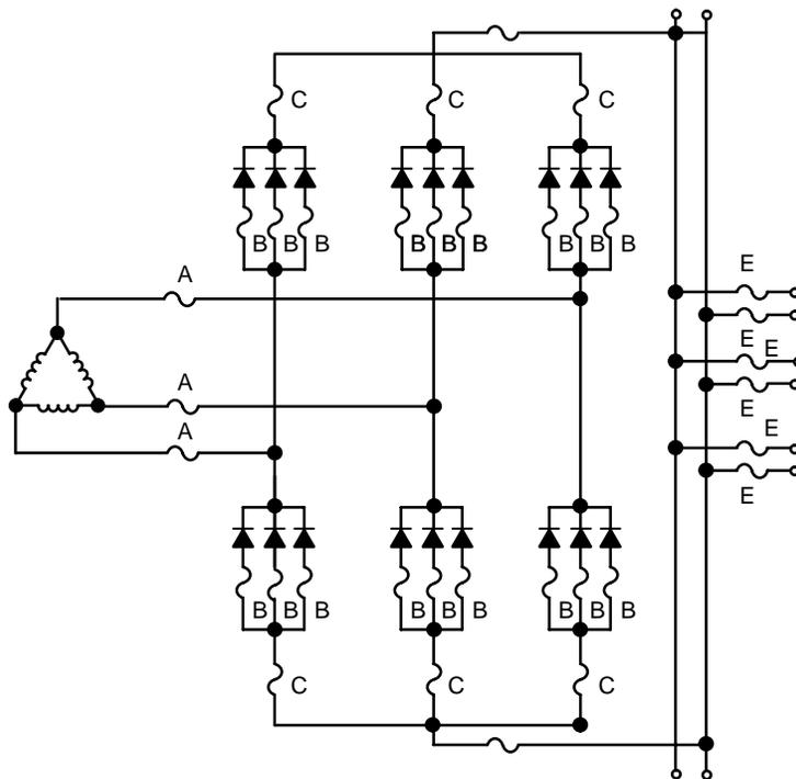
Figure 149. Fuse Placements in a Redundant System
