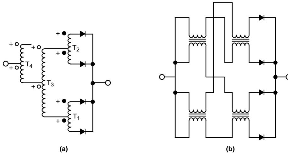
**Figure 100. Schemes for Balancing the Current When More than Two Diodes are Required.**
