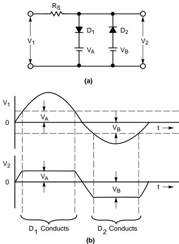
**Figure 155. Diode Clipping Circuit and Waveforms when Peak Clipping a Sine Wave:**
