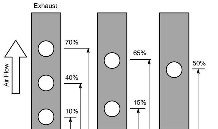
**Figure 215. Proper Rectifier Placement for Components having Equal Power Dissipation. Located in this fashion, each semiconductor will operate at the same case temperature and maximize the heatsink performance. In natural convection, mounting must be vertical.**
