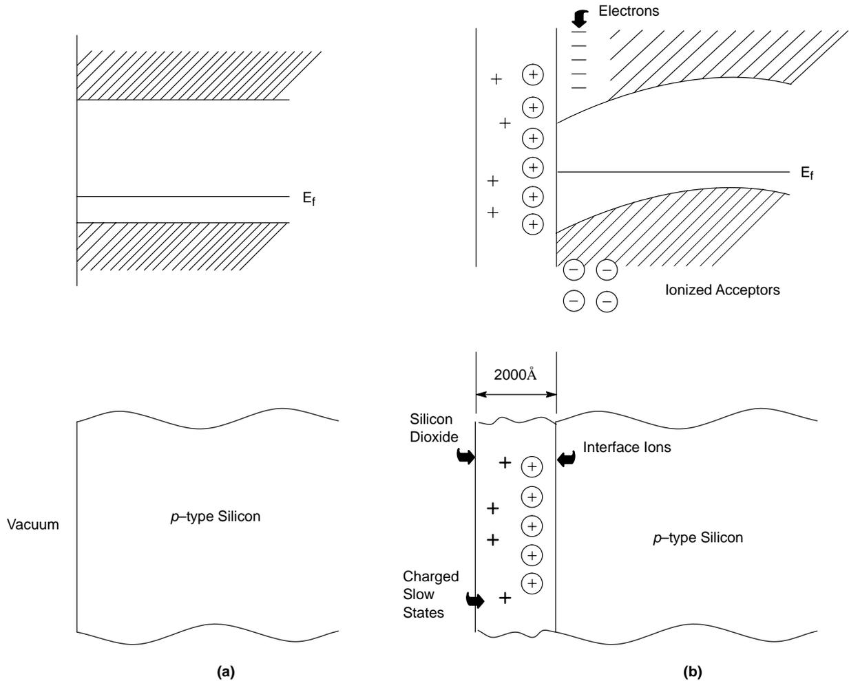
Figure 11. (a) Ideal Surface; (b) Band Bending Due to Energy States in the Forbidden Energy Gap
