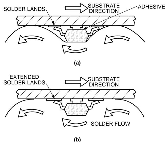
**Figure 221. Shadowing in Wave Soldering: (a) Surface Tension and Body Height Can Prevent Molten Solder Reaching the Downstream End of the SMD, the “Shadow Effect”; (b) Extending the Solder Land May Overcome Shadowing**
