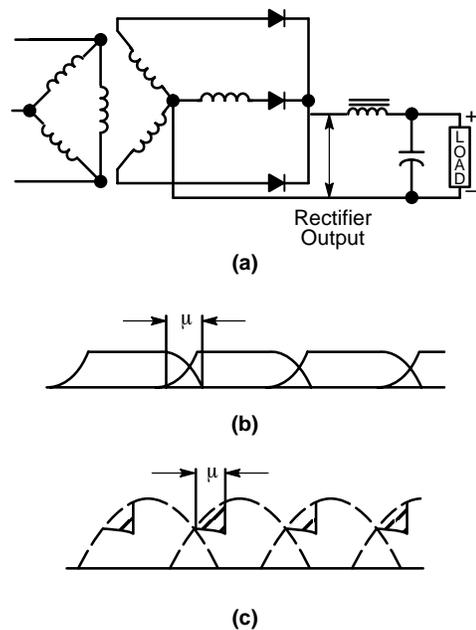
**Figure 104. Effect of Transformer Leakage Inductance on the Behavior of a Polyphase Rectifier:**
