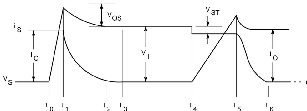
Figure 178. Power Switch Waveforms for the Buck Converter
