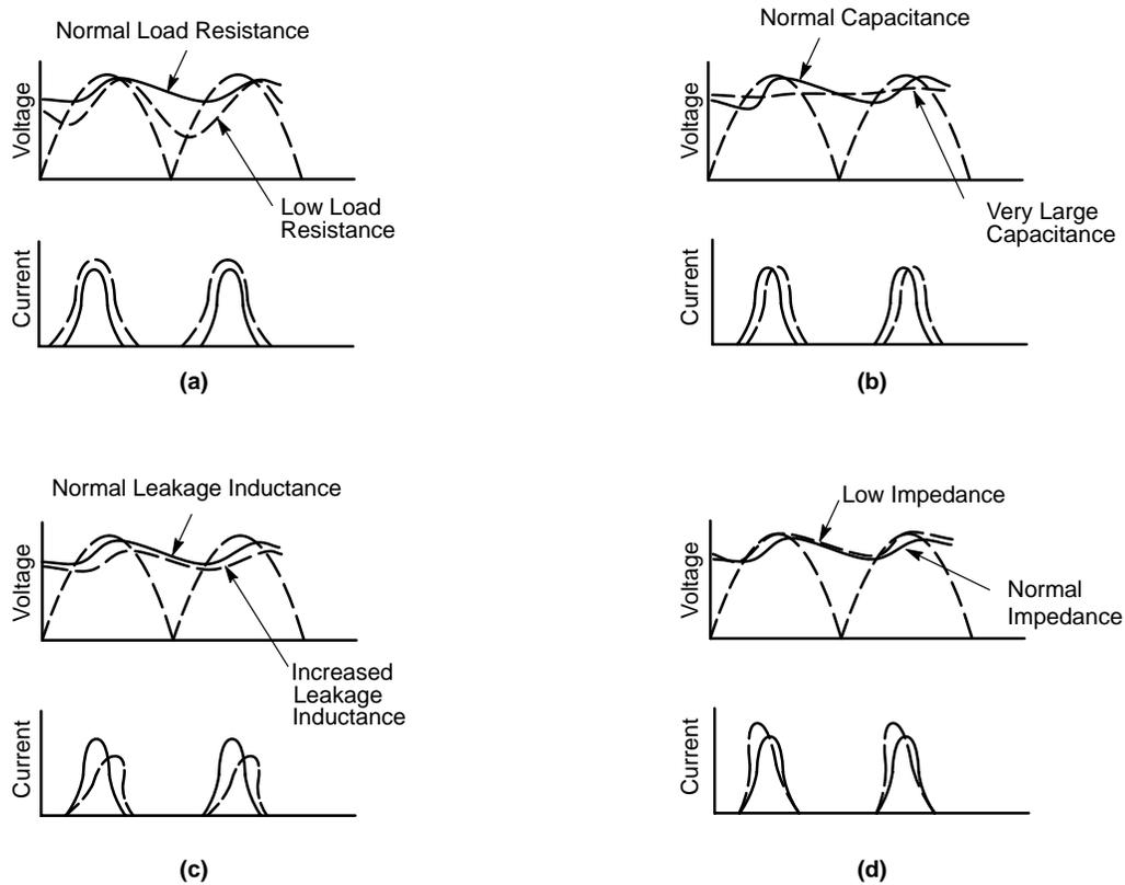
**Figure 106. Effects of Circuit Constants and Operating Conditions on Behavior of Rectifier Having a Capacitor-Input Filter: (a) Effect of Load Resistance; (b) Effect of Capacitance; (c) Effect of Transformer Leakage Inductance; (d) Effect of Very Low Diode and Transformer Impedance**
