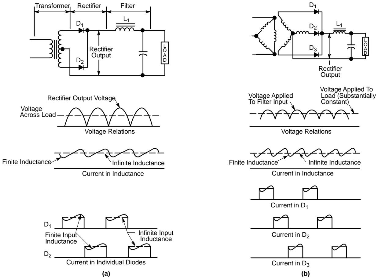
**Figure 101. Voltage and Current Waveforms Existing in Rectifier Systems Operating with Choke-Input Filters:**
