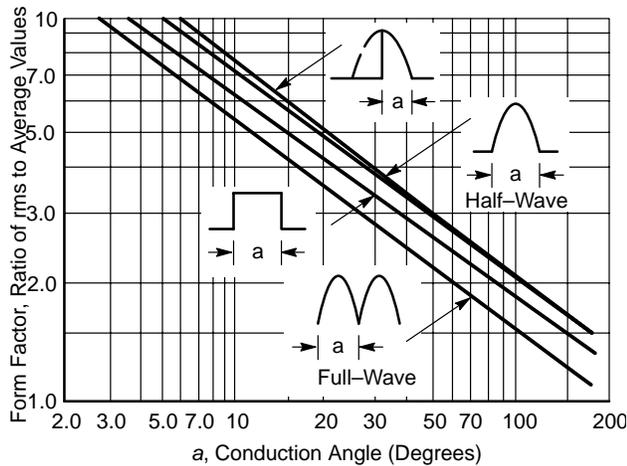
Figure 75. Form Factor for Various Current Waveforms
