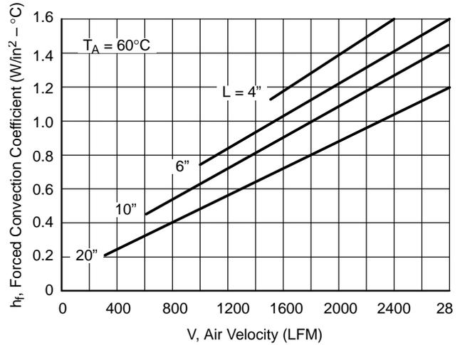
Figure 202. Heat Transfer Coefficient for Forced Air Convection
