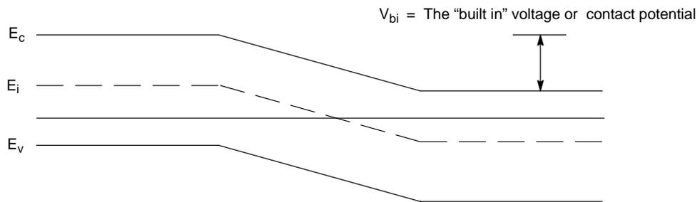
Figure 13. Band Diagram of Ideal Pit Junction
