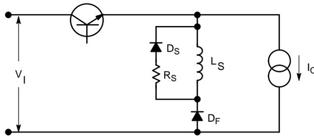
Figure 180. Buck Converter with Dissipative Turn-on Snubber
