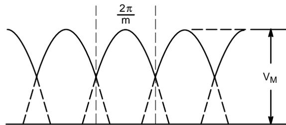
**Figure 92. Rectified Voltage Waveforms for Multiphase Rectifier Circuit. The number of output pulses per cycle is designated**
