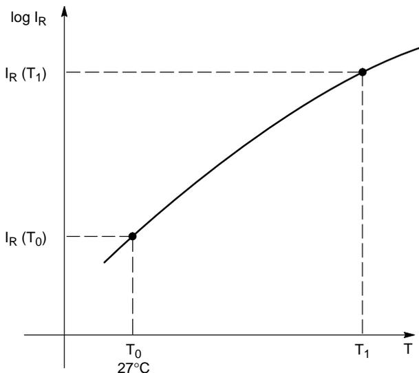
Figure 63. Typical Reverse Leakage Current Temperature Characteristics
