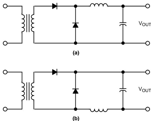
**Figure 166. Output Rectifier Configurations:**
