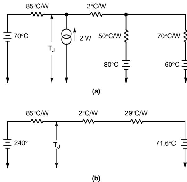
**Figure 35. Successive steps in the solution of the example in the text. Thermal problems may be solved by applications of network theorems. (a) Model with example numbers inserted; (b) Simplified thermal circuit obtained by applying Thevenin's Theorem to each side of the model**
