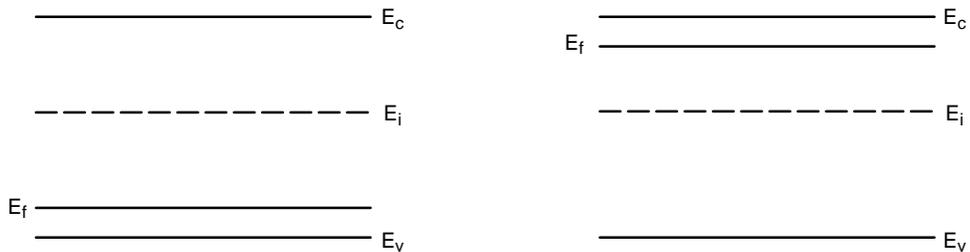
Figure 12. Band Diagram Prior to Junction Formation
