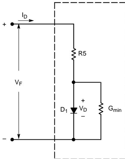
**Figure 48. DC Large-signal SPICE Diode Model**
