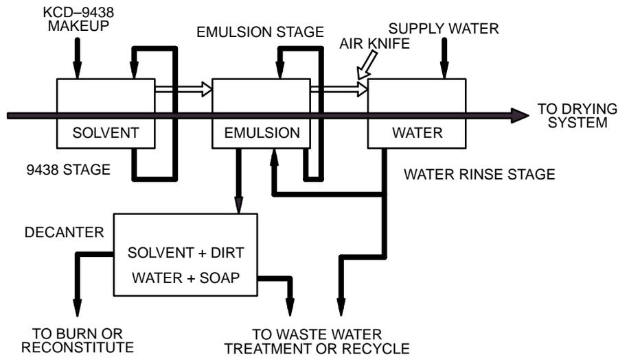
Figure 222. Semiaqueous Cleaning System (courtesy of Du Pont)
