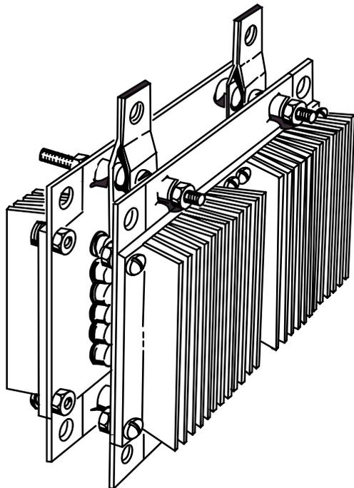
**Figure 213. A 650 A Rectifier for 3–Phase Service Having Integral Heatsink Designed for Forced Air Systems**
