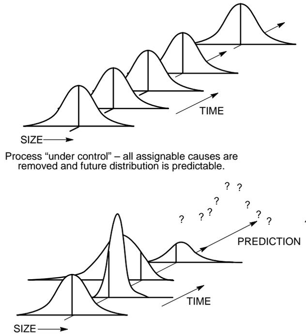
**Figure 197. Impact of Assignable Causes on Process Predictability**
