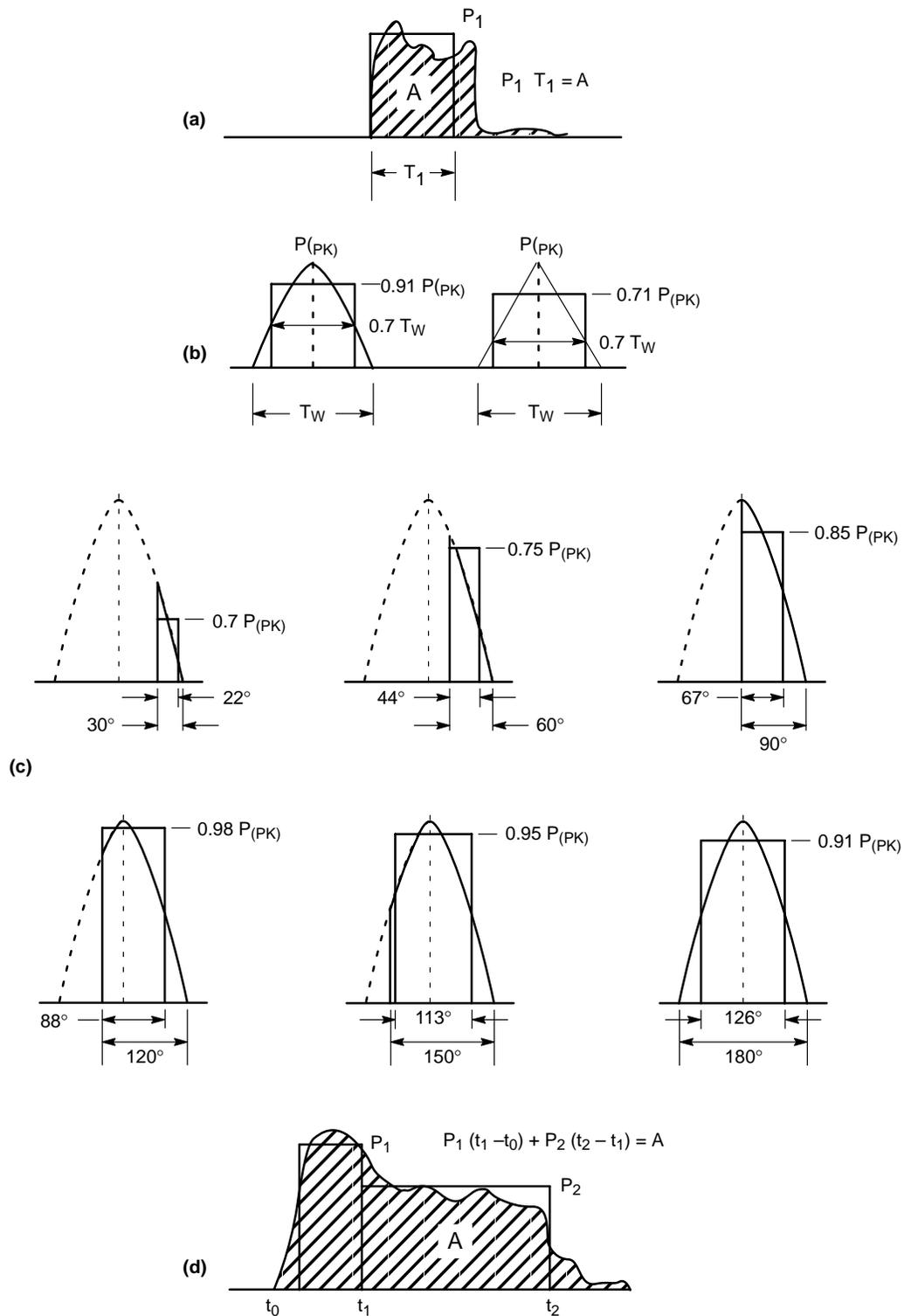
**Figure 42. Models for Frequently Encountered Power Pulses**
