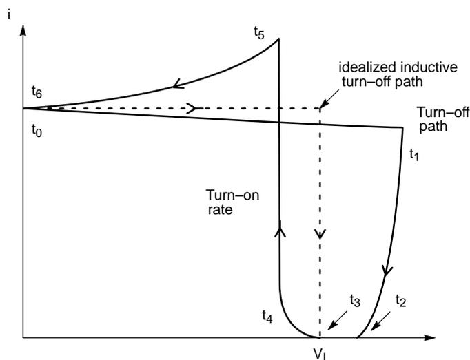
Figure 179. Switching Load Loci for the Buck Converter
