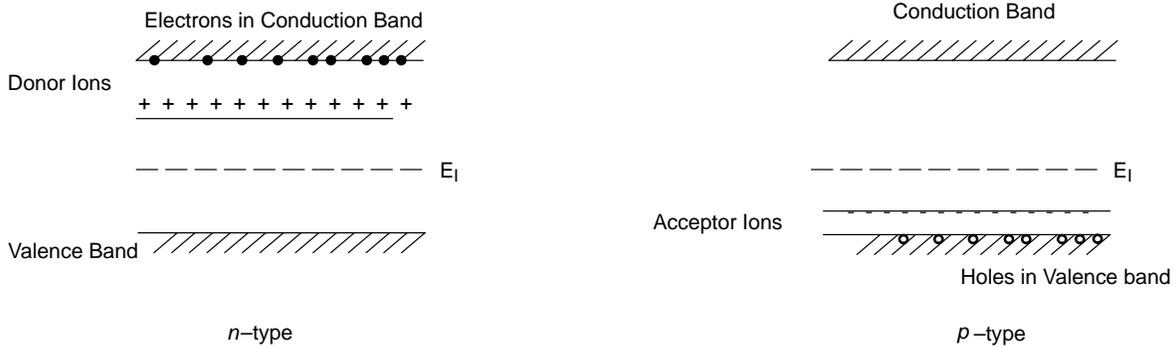
Figure 5. Band Diagram for n-type and p-type Semiconductors
