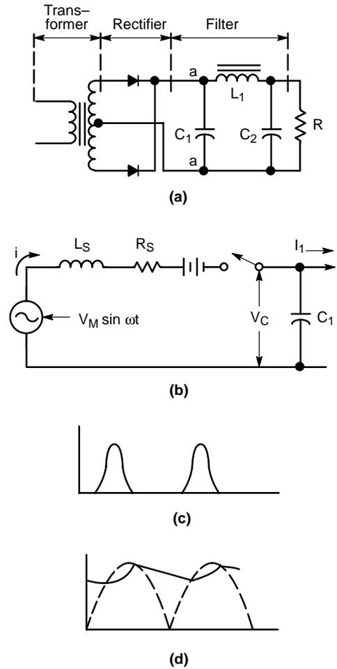
**Figure 105. Actual and Equivalent Circuits of Capacitor-Input Rectifier System, Together with Oscillograms for Voltage and Current for a Typical Operating Condition:**
