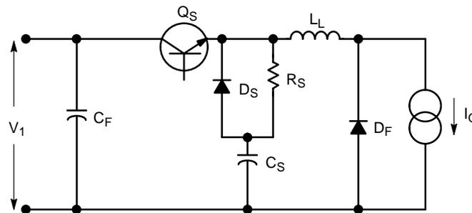
Figure 182. Buck Converter with Dissipative Turn-off Snubber
