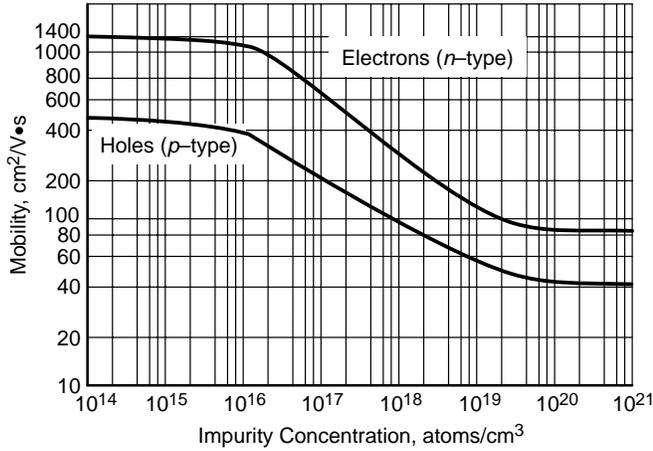
Figure 7. Bulk Mobility Versus Doping for Silicon
