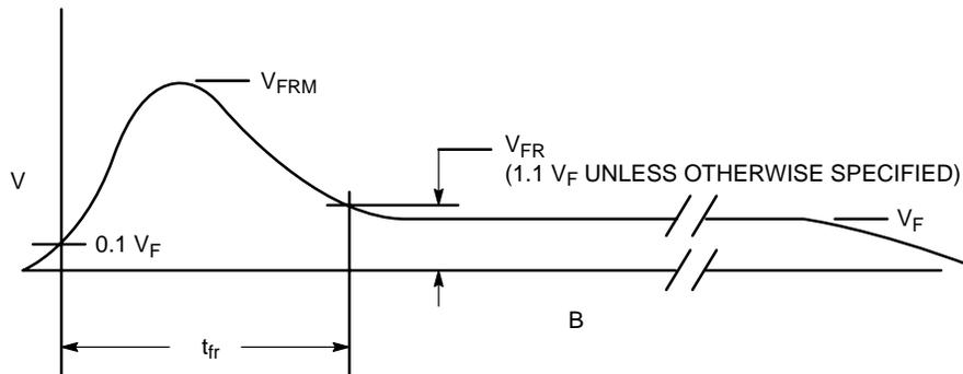
Figure 85. Turn-on Waveform Showing JEDEC Defined Terms.
