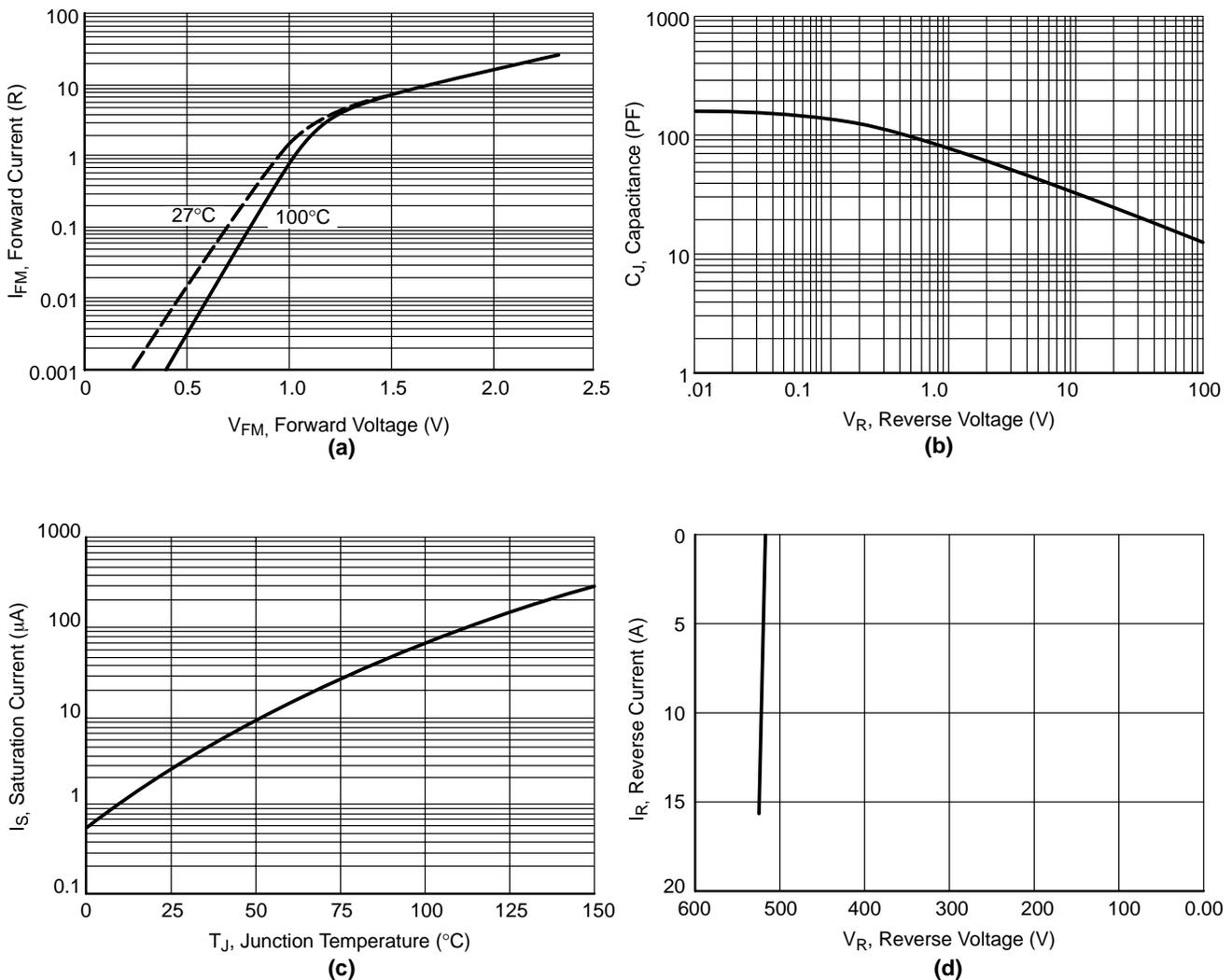
**Figure 70. (a) MURH840CT SPICE Model Forward Voltage DC Characteristics at 27°C and 100°C;
