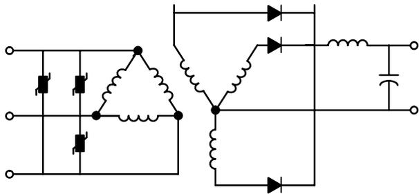
Figure 141. Transient Suppression in a Three-Phase Rectifier
