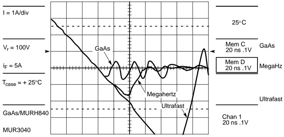
**Figure 28. The Reverse Recovery Characteristic of Ultrafast, Megahertz and GaAs at  $T_A = 125^\circ\text{C}$ . All Devices Exposed to the Same Test Conditions.**
