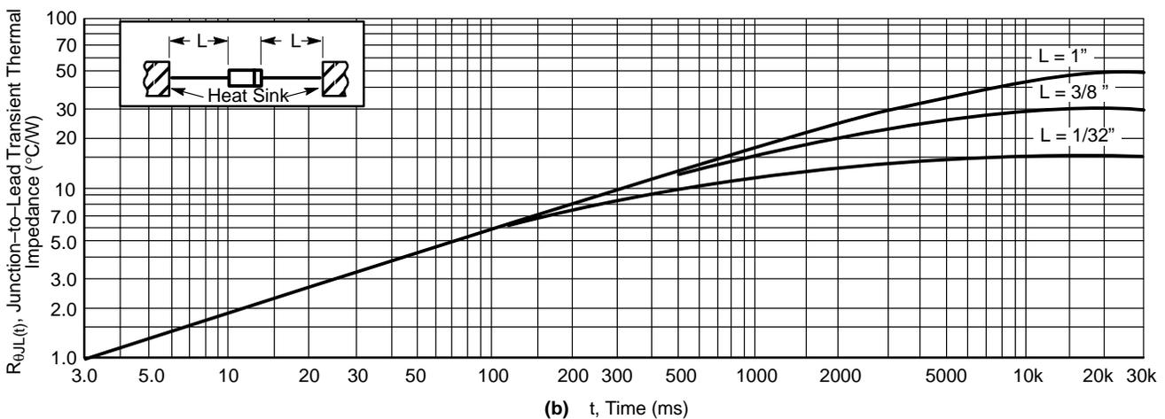
**Figure 38. Typical Thermal Response of Lead-Mounted Rectifiers**
