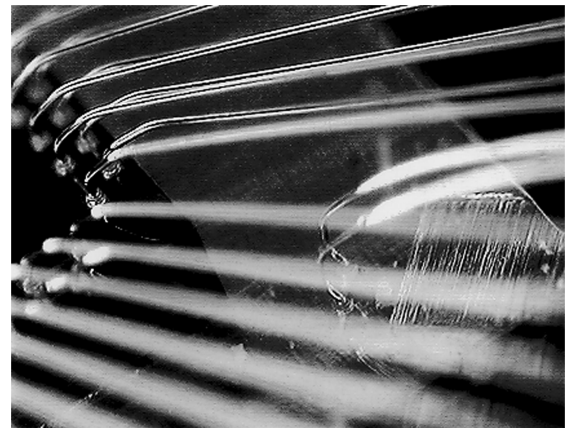
FIGURE 3. 60 micron Staggered Fine Pitch Wire Bonding Capability
