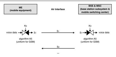
**Figure 13.14** Data transmitted between the mobile station and the base station via the air interface are encrypted using the A5 cryptographic algorithm and the secret key Kc. This process must be preceded by authentication of the SIM by the GSM background system
