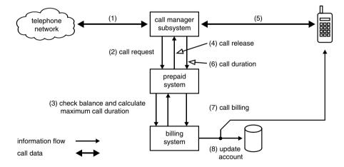
**Figure 13.21** Basic architecture of a system for prepaid SIMs using the SICAP Prepaid Roaming solution as an example. This diagram shows the progress of a call made to a mobile telephone, with the numbers in parentheses indicating the sequence of events. The call management subsystem is part of the GSM background system, and may for example be a component of the mobile switching center (MSC)
