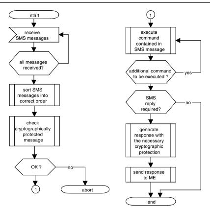
**Figure 13.20** Flow chart of the basic program sequence for remote file management (RFM) via the air interface using OTA, as specified in GSM 03.48. Remote file management is essentially performed by the processes shown in the upper right branch of the flow chart, with the remainder of the processes serving to establish secure communications in accordance with GSM 03.48
