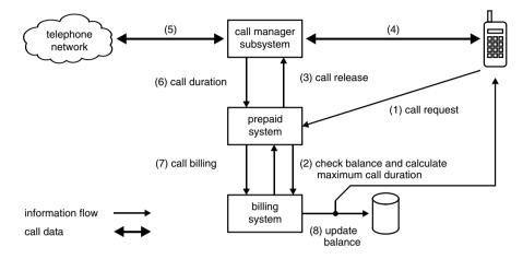
**Figure 13.22** Basic architecture of a system for prepaid SIMs using the SICAP Prepaid Roaming solution as an example. The diagram shows the progress of a call originating from the mobile telephone, with the numbers in parentheses indicating the sequence of events. The call management subsystem is part of the GSM background system, and may for example be a component of the mobile switching center (MSC)
