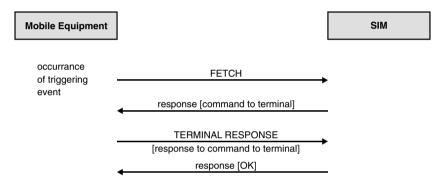
**Figure 13.17** The extended protocol process between the mobile equipment and the SIM for the proactive commands of the SIM Application Toolkit, as specified in GSM 11.14. The response of the smart card to a command contains a command to the terminal in the data part. The terminal executes this command and returns the associated response to the smart card in the data part of a command. The sequence shown here is based on the transmitted APDUs and shows only successful results
