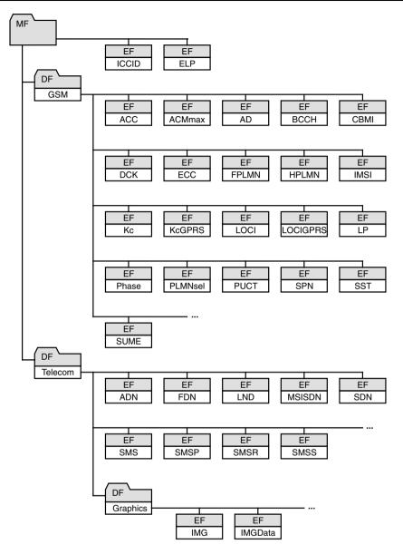
Figure 13.12 Overview of the most important SIM files
