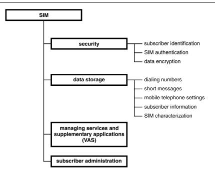
Figure 13.10 Classification of the basic functions of the SIM in the GSM system
