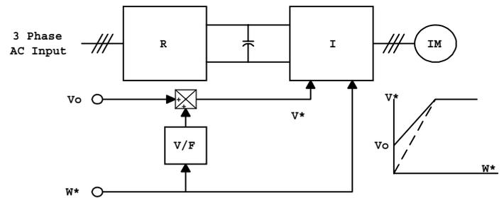
Fig. 7 Open loop volts/hertz control
