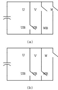
Fig. 3(a) shows that the inverter switching state for the period  $T_1$  for vector  $V_1$  and Fig. 3(b) is for vector  $V_2$ , resulting switching patterns of each phase of inverter are shown
