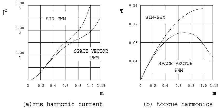
Fig. 6 Current and torque harmonics
