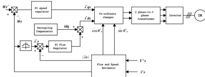
Fig. 9 Block diagram of sensorless vector control system.
