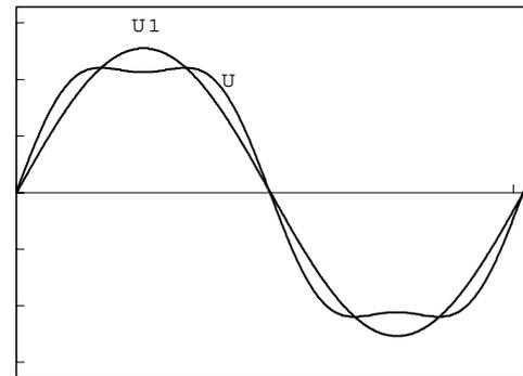
Fig. 5 Phase-to-center voltage By space vector PWM
