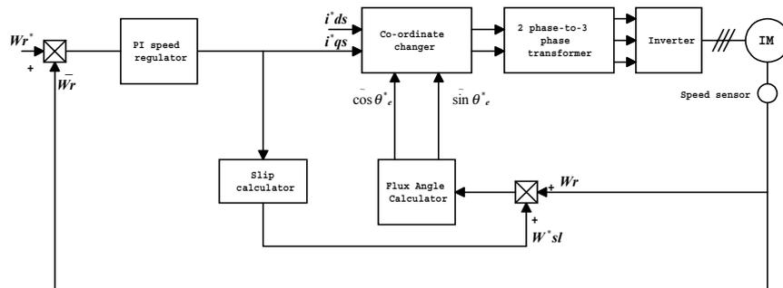
Fig. 8 Block diagram of vector control system with speed sensor.
