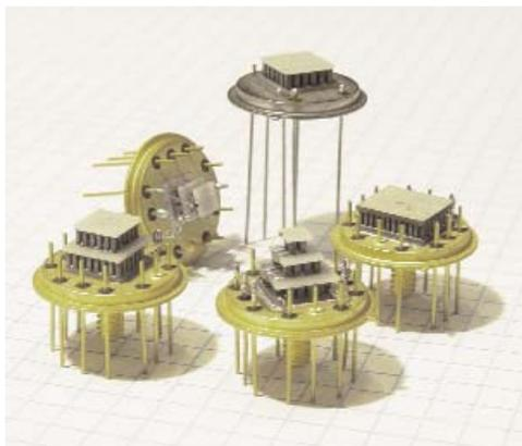
Figure 9.1.2.2. Examples of mounting by soldering on the TO8-style headers
