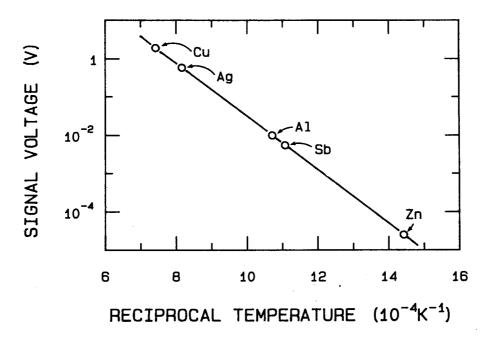
Fig. 10.1: Relationship between signal voltage of an infrared radiation thermometer and reciprocal temperature after calibration at five metal freezing points [after Sakuma and Hattori (1982b)].
