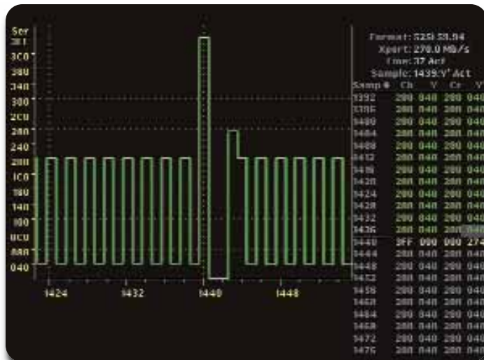
► Figure 29. 270 Mb/s EAV timing reference packet viewed as multiplexed data.
