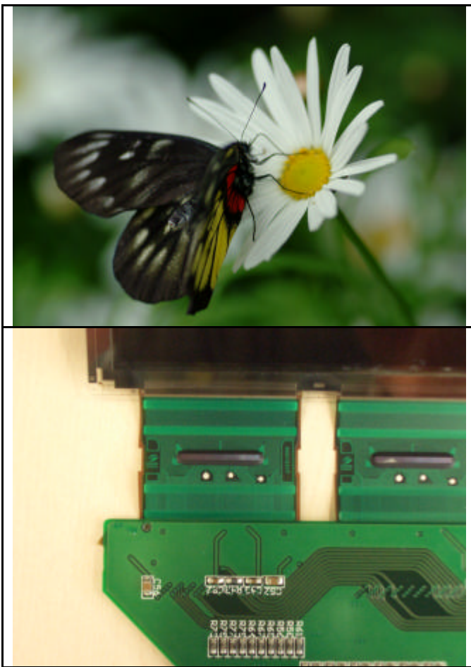
Fig. 3a,b SXGA Panel output by using SSD1231 source driver
