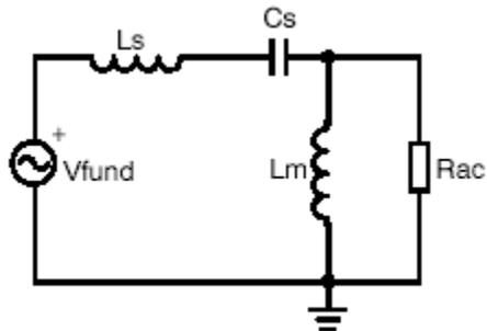
Figure 3: Substitutive schematic of the LLC resonant converter
