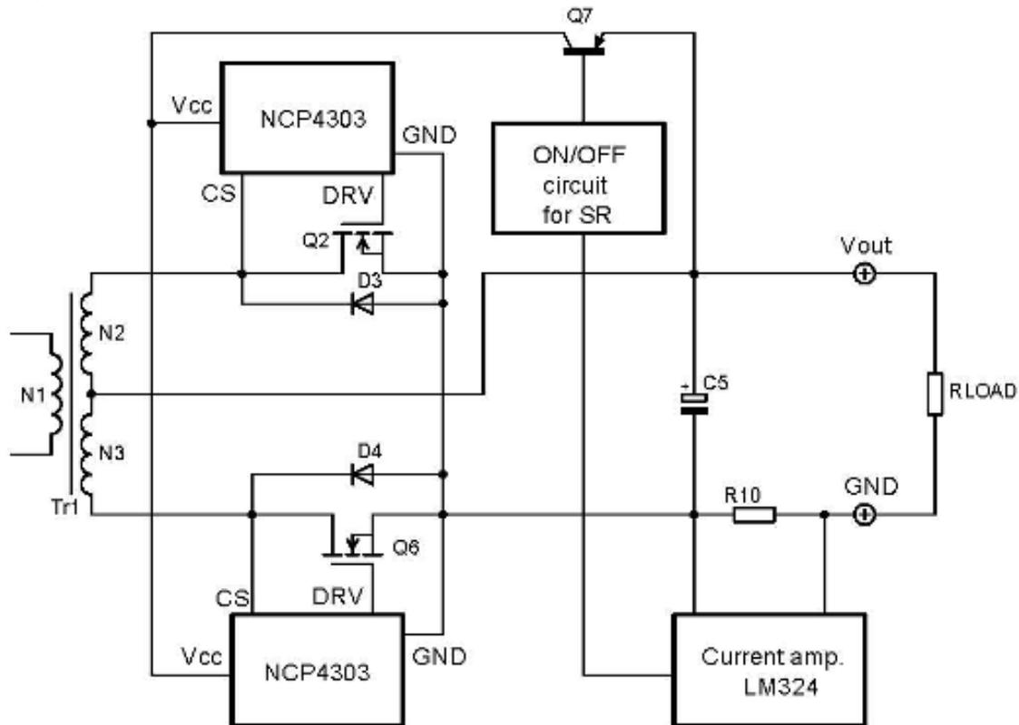
Figure 6: Syn. Rectification controller is shut down when the output current is low
