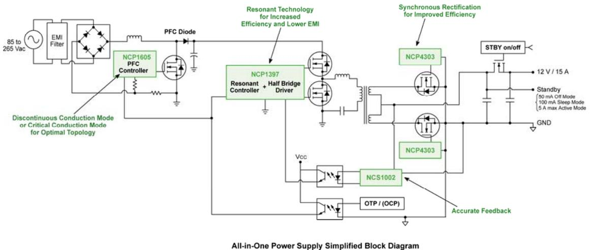
**Figure 1: Reference Design Architecture Simplified Block Diagram**
