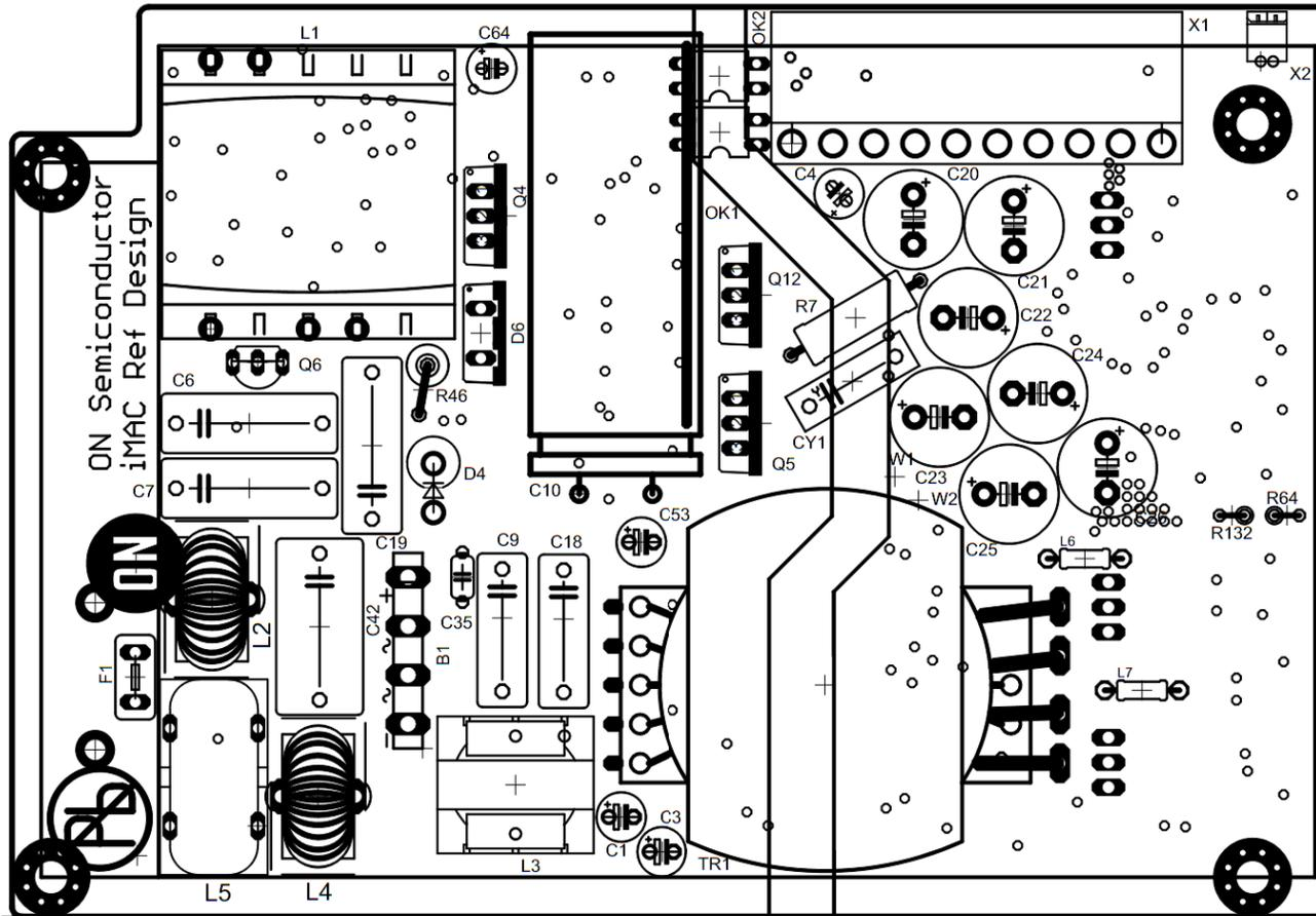
Figure 13: Top side components
