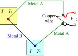
connected to the positive terminal of the DMM, and the other is connected to the negative terminal so that the measured voltage increases with increasing temperature.
