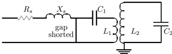
Figure 3: Tesla Circuit With Gap Shorted.
