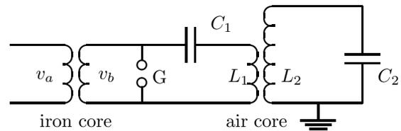
Figure 1: The Classical Tesla Coil
