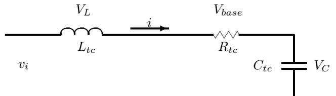
Figure 8: Tesla Coil with Series Resonant LC Circuit
