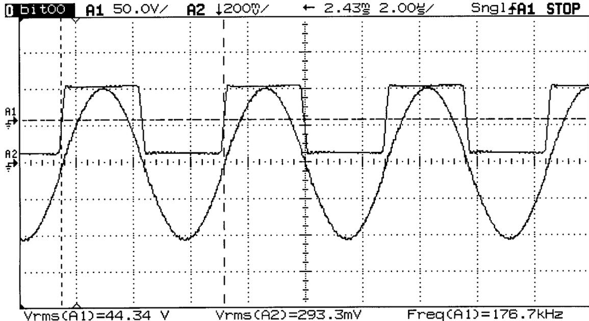
Figure 12: Square wave of voltage, sine wave of current at base of coil 12T below breakout.
