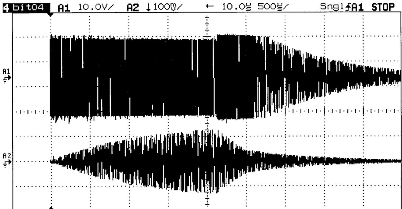
Figure 13: Tesla Coil Voltage and Current Waveforms
