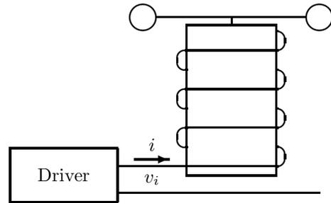
Figure 7: Drive for Tesla Coil
