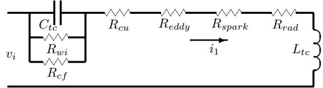
Figure 11: Detailed Lumped Model of Tesla Coil
