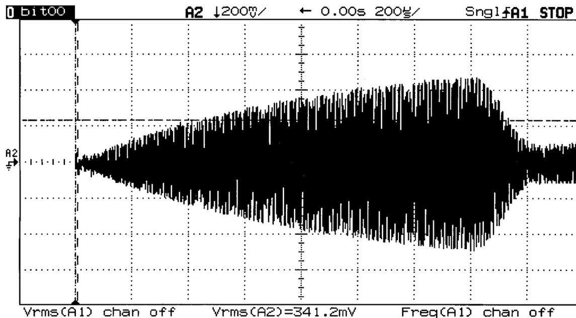
Figure 14: Current Waveform with Voltage =  $\pm 604$  V
