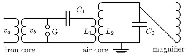
Figure 6: The Classical Tesla Coil With Extra Coil
