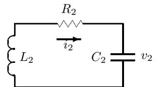
Figure 5: Lumped Circuit Model Of A Tesla Coil, arc off.
