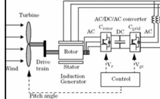
The ac/dc/ac converter consists the rotor-side converter (Crotor) and the grid-side converter (Cgrid). Both Crotor and Cgrid converters are voltage-sourced converters using forced commutated power electronic
