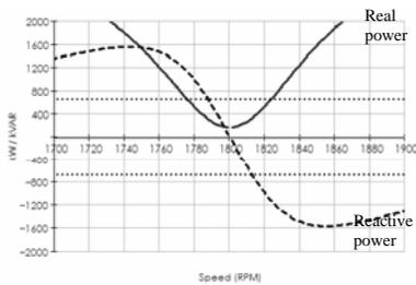
Variation of the real (solid red) and reactive (dash blue) power with the slip for a squirrel-cage induction generator
