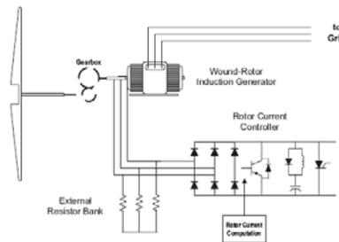
Wind turbine electrical generator with variable slip control
