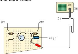
Then adjust the timebase, CH1 Volts per division, Chi pos and trigger settings until something like this appears.
