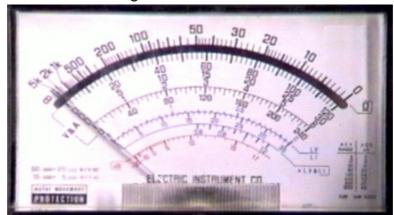
Here on the second scale the minor divisions are 1/8 th of a large division. The meter range can be set to 6V, 30V, 120V, 240V and so the resolutions are:
