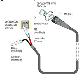
Then connect to the circuit as required, the Red lead to the test point, the back lead to zero volts.
