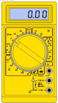
When using a DMM it is important to realise the significance of resolution. Generally DMM have what are known as 3  $\frac{1}{2}$  digits displays. That is they can display numbers in the range  $\pm 1999$ , where the decimal point can be moved. Usually giving ranges of 20mV, 2V, 20V, 200V etc
