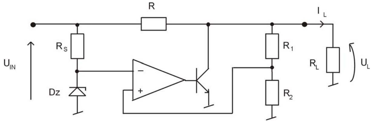
One important advantage of the shunt regulator is that it is not damaged by a short – circuited output. The short – circuit current is limited to  $U_{IN}/R$  and provided the power rating for the resistor  $R$  is sufficient to withstand the short – circuit current, then there is no damage.
