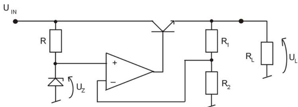
In this circuit the Zener voltage is more stable because the variation of the load current does not affect the Zener current. In addition, the large loop gain, resulting from the op amp, ensures that very small changes of the output voltage are detected and rapidly corrected.
