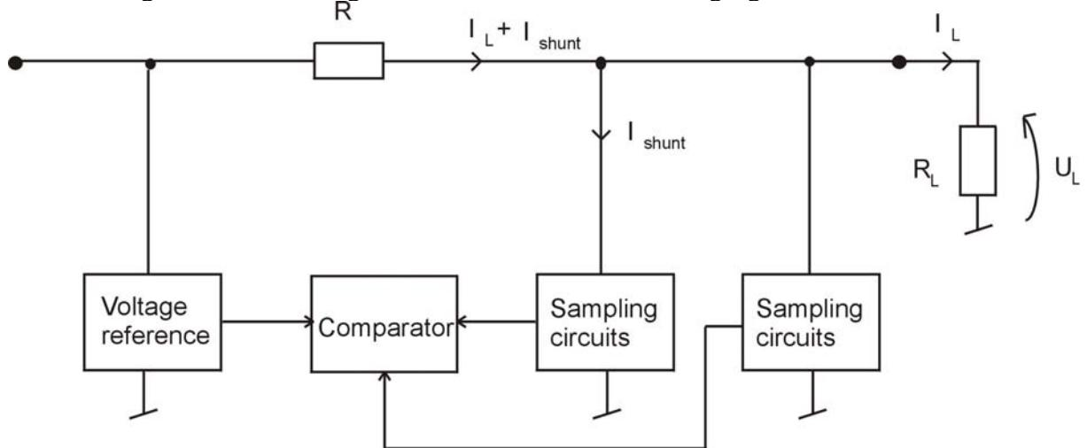
As for the series regulator the current through the control element is determined by the output voltage sample which is applied to the comparator.
