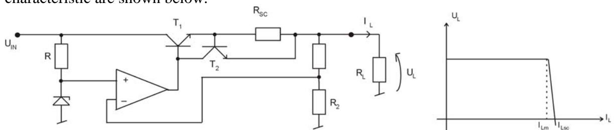
When  $U_{BE2} = I_L * R_{SC}$  reaches  $U_{BEF} = 0.7V$   $T_2$  begins to conduct heavily and consequently current which should be flowing into the base of  $T_1$  is diverted to the collector of  $T_2$  and thus  $T_1$  is protected. The current through  $T_2$  is limited by the current sourcing capability of the operational amplifier, which may be a few tens of mA.
