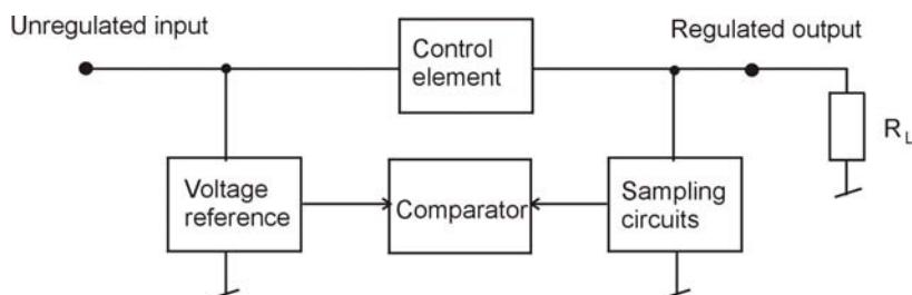
Control is achieved by comparing the required output with a fixed voltage reference. If the output voltage changes, for example as a result of a variation in the load current, the input to the comparator from the sampling circuit changes in the same direction. The output generated by the comparator, resulting from the error signal, causes the control element to vary the
