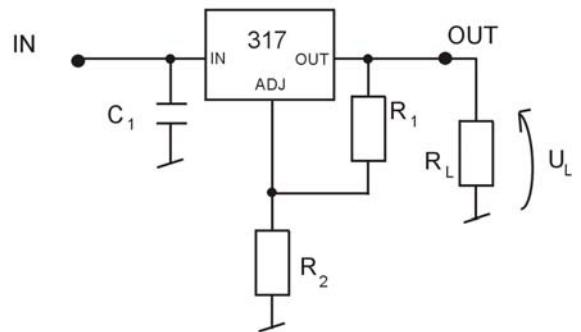
This regulator has no GROUND terminal. It adjust  $U_{OUT}$  to maintain a constant voltage of  $U_{REF}$  ( $U_{REF} = 1.25$  for LM317) between the output terminal and the adjustment terminal. It can be easily shown that the output voltage is:
