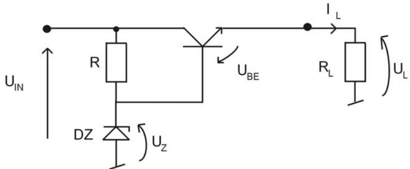
The comparator function is performed by the base emitter junction which controls current flow through the transistor.
