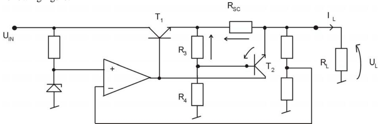
The circuit is similar to the basic, current – limiting circuit except that the base of T<sub>2</sub> is taken to a potential divider comprising R<sub>3</sub> and R<sub>4</sub>. The base – emitter voltage of T<sub>2</sub> is:
