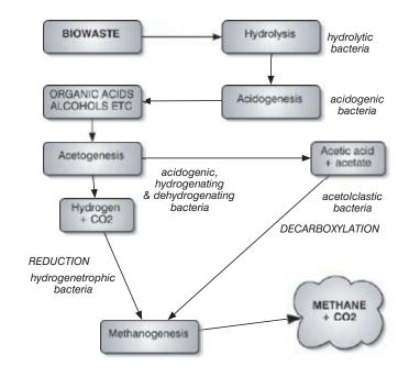
Figure 2 Flowchart indicating the main stages in Anaerobic Digestion Source: Evans G, Biowaste and Biological waste treatment 2001
