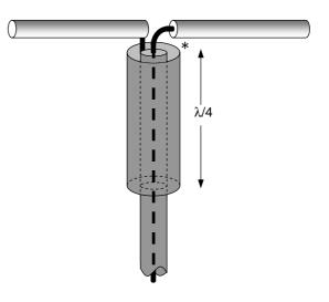
terminals. I'd expect that if the terminal of the dipole limb connected to the co-axial inner conductor were also connected to the sleeve where I've shown an asterisk this would form a co-axial Pawsey stub, but I've never seen this applied in practice.
