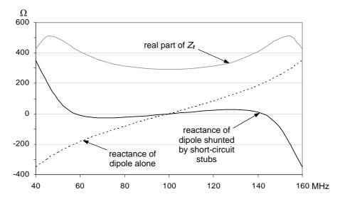
Thus the 'reactance compensation' effect of the short-circuit stubs is demonstrated although, in practice, the result may not be so smoothly-changing or so symmetrical. Also, this shouldn't be interpreted as meaning such a folded dipole can be operated over 70 to 130 MHz, or more, because variation of  $R_r$  and other factors neglected in the simple model would limit the usable bandwidth.
