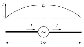
standard text books on antennas state that this is supported by experimental results. In many respects a centre-fed dipole behaves like a balanced transmission line, open circuit at the far end(s), so a voltage applied (or induced) at the terminals gives rise to a standing wave which must have zero current at the open-circuit ends. Assuming a simple sinusoidal current distribution, the result would be as illustrated to the left. Note that the currents in both
