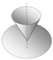
A bit of imaginative manipulation of the two apex angles leads to the idea of an infinite 'discone' where the apex angle of the outer cone has been increased to 180° making this conductor an infinite disc. I've drawn a truncated section of this to the left. Of course, the 'ratio of diameters' becomes meaningless in this case.
