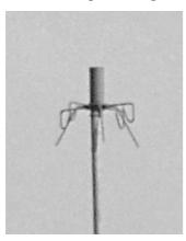
The manufacturer from whom I borrowed the antenna pictured above once told me these are referred to as 'discones' by the Admiralty. The design has lasted well but now it appears it is being displaced by a ground-plane type of antenna, the Racal Antennas RA978 [85] consisting of a "fat" folded monopole above four sloping and four non-sloping radials, the latter formed into loops, wrought-iron fashion, as shown to the left – I haven't yet managed to figure that one out!
