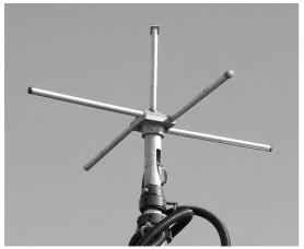
Two well-known practical implementations are the VHF/UHF 'ground plane' antenna, shown to the left using skeletal radial rods ( $\geq \lambda/4$  long), and the medium-wave transmitting antenna using a guyed lattice mast and wire 'radials' buried in the earth. Sometimes the monopole element is folded to increase its radiation resistance, which may simplify matching.
