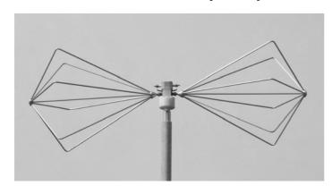
We have a cage biconical dipole in Spectrum Planning Group, shown to the left, built in-house for early EMC measurements. The terminals of the dipole limbs are connected to a balun (the small box in the middle) by rather long copper straps and its performance is not as good as would be hoped. The converging cones at the ends of the limbs may be a convenient way to prevent this item of laboratory equipment potentially "poking one's eye out" rather than having significant electrical properties.
