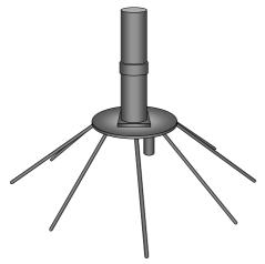
has the effect of increasing the terminal resistance and reducing the angle of elevation of the VRP lobe. A particularly interesting example is the AS-390/SRC military UHF communications antenna [69], [70], illustrated to the left, which also has the down-lead connected part way up the monopole via a short-circuit stub.
