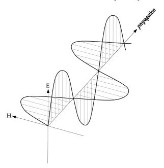
related by Z, the intrinsic impedance of the propagating medium (see the box below: the intrinsic impedance of space). For simple antennas, the transition into the far field occurs at a distance from the antenna  $r > 2\pi\lambda$ , where  $\lambda$  is the wavelength in use.
