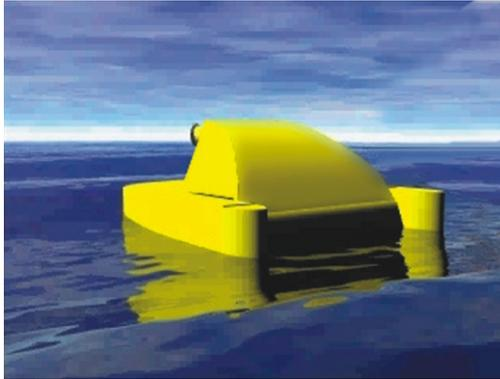
The main prototype device for moderate water depths (i.e up to ~20 m) is the **OSPREY**<sup>19,20</sup>, developed by Wavegen Ltd. in the UK. It is designed for deployment on the seabed. A 2 MW prototype is planned, which will operate in 15m depth within 1 km from the shore.
