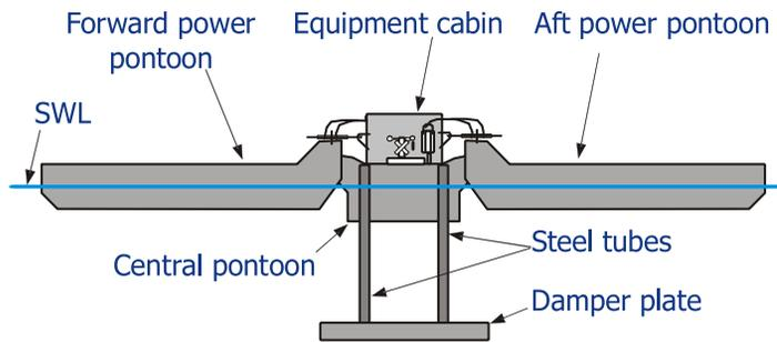
The **McCabe Wave Pump**<sup>23,24</sup>, consists of three rectangular steel pontoons, which are hinged together across their beam. The bow of the
