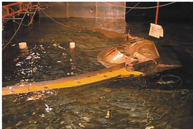
higher-level reservoir. Electricity is produced by a set of low-head Kaplan turbines. The scheme has been tested in the laboratory at 1:50 scale and on a 1:3.5 scale model turbine. A 57 m wide and 261 tons heavy prototype in scale 1:4.5 rated in full scale to 4 MW is being deployed in Nissum Bredning, Denmark.
