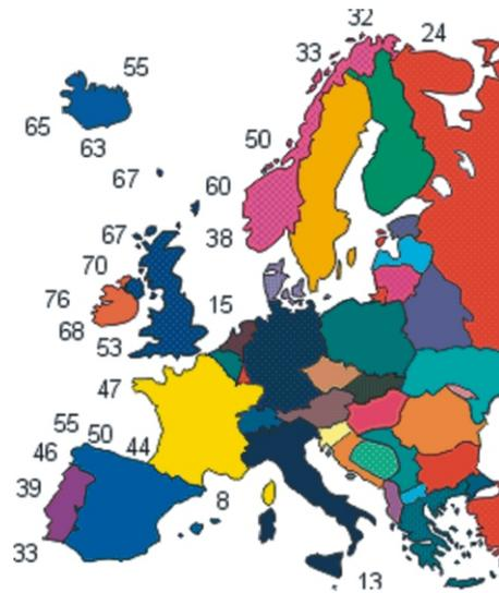
**Figure 2:** Wave power levels in kW/m of crest length in European waters.
