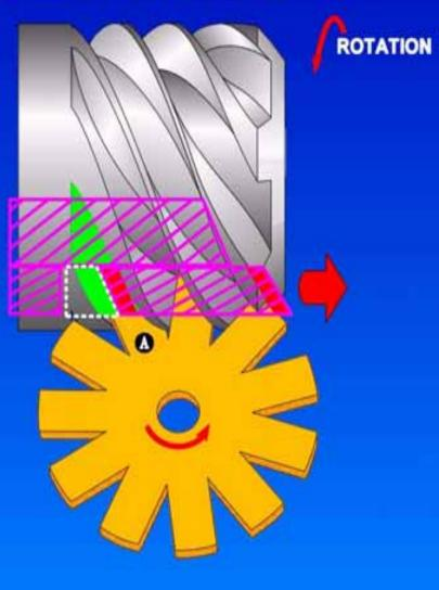
**Rotary Screw Compressor Capacity Control**  <u>Electronic Capacity Control</u> – VFD Drive (Speed Control) Internal Leakage in Compressor Increases at Slower Speeds Mechanical Capacity Control
