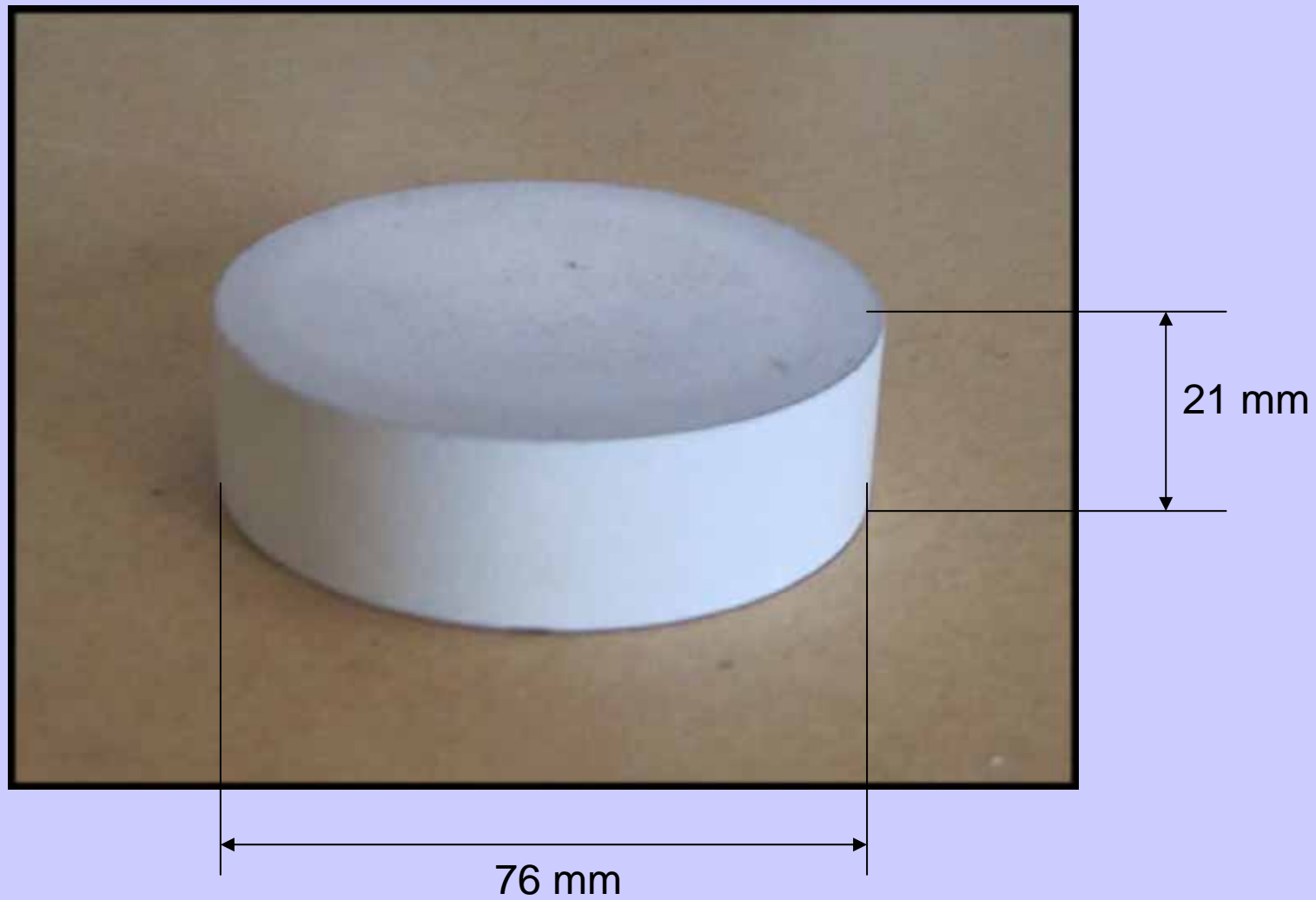
ZnO-varistor-disk, U_{(10 \text{ kA})} = 6 \text{ kV}
