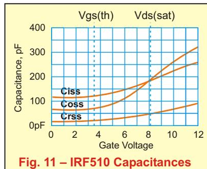
Fig. 11 – IRF510 Capacitances
