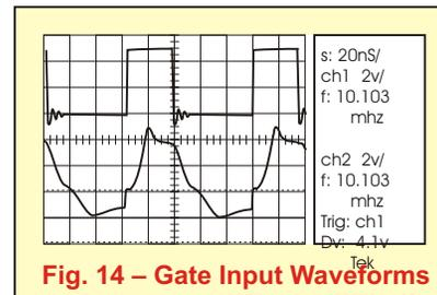
Fig. 14 – Gate Input Waveforms
