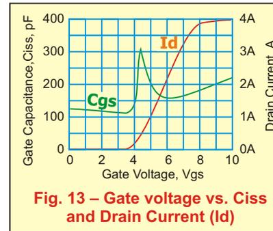
Fig. 13 – Gate voltage vs. Ciss and Drain Current ( $I_d$ )
