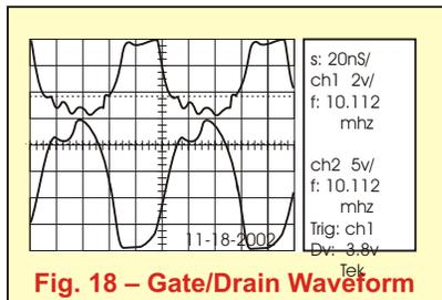
**Fig. 18 – Gate/Drain Waveform**
