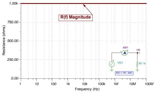
**Fig. 1.9: Intuitive Resistor Model**
