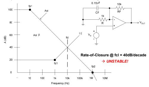
Fig. 1.21: Loop Gain Stability Example
