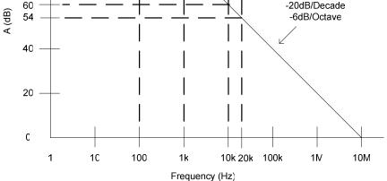
Fig. 1.4: Magnitude Bode Plot: 20 dB/Decade = 6 dB/Octave
