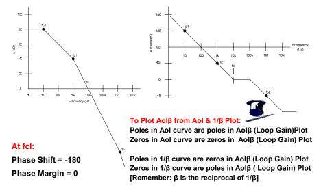
Fig. 1.22: Loop Gain Plot From Aol Curve & 1/β Plot
