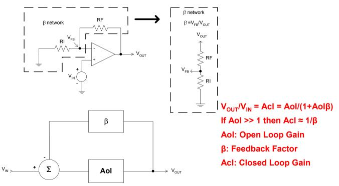
Fig. 1.14: Op amp Loop-Gain Model
