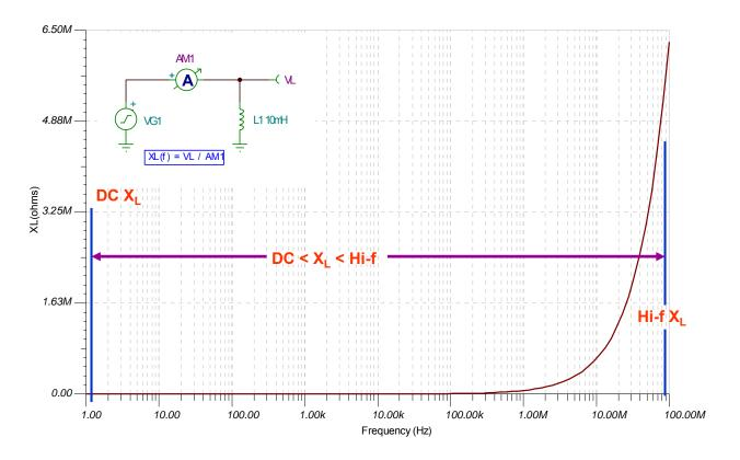
Fig. 1.13: Intuitive Inductor Model SPICE Simulation
