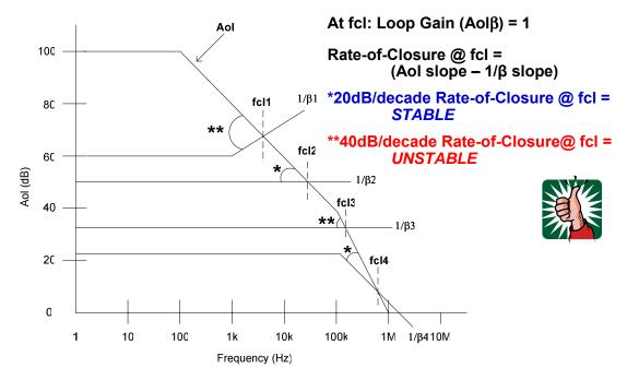
Fig. 1.20: Rate-Of-Closure Test for Loop Gain Stability
