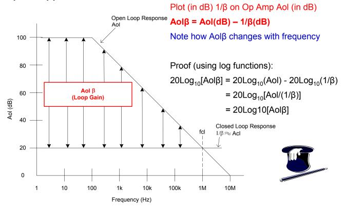
Fig. 1.19: Loop Gain Information From Aol Plot And 1/β Plot
