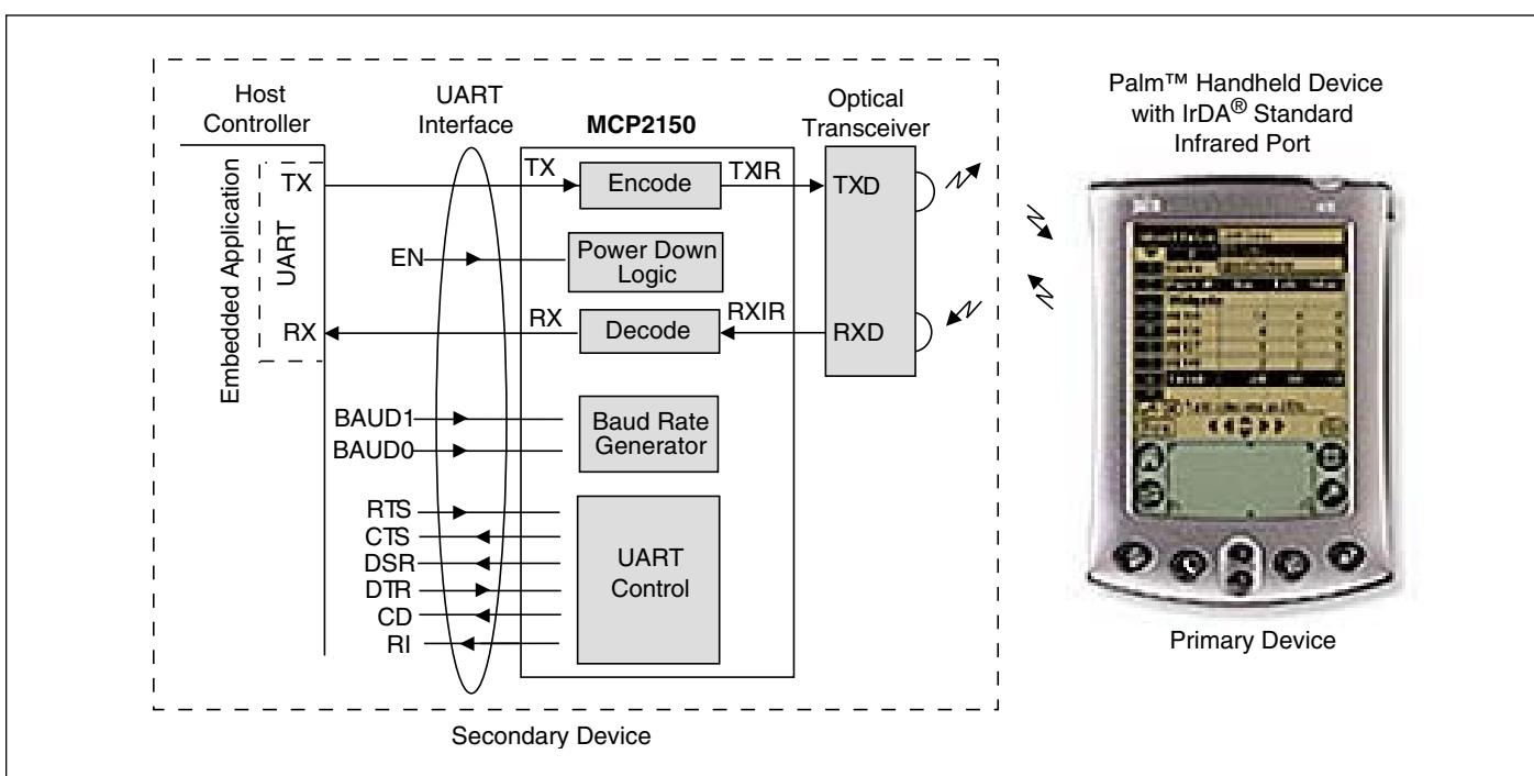
**Figure 1.** The Primary Device (PDA) sends data through the infrared interface to the MCP2150. The MCP2150 then decodes this data into the UART standard. After translation, the data is sent to the Host Controller through the UART interface. The Host Controller can also send data to the MCP2150 where the data is encoded and made ready for transmission to the Primary device.
