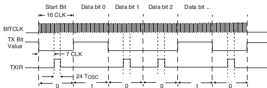
**Figure 4.** Bit Encoding
