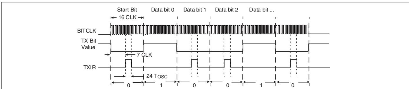
**Figure 4.** Bit Encoding
