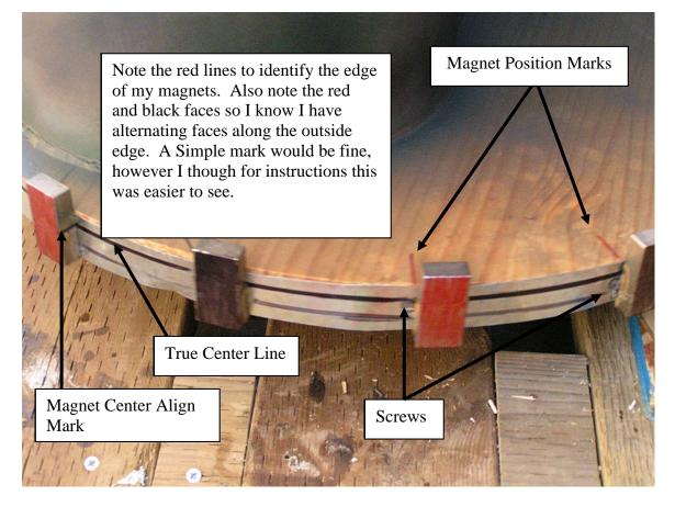
**Step 3**: Attach flashing around the edge of the rotor. Put a screw in a starting point that is fairly centered between your magnet position marks. Work your way around the whole
