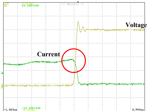
Figure 24. Typical hard switching turn-off waveforms. High voltage and high current occur at the same time.
