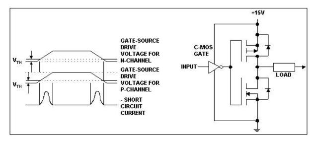
Figure 5. P/N-Channel HEXFET Power MOSFET Totem Pole with Drive Circuit for Operation at Low Voltages
