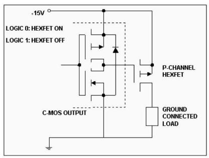
Figure 2. Switching Ground-Connected Loads Operating from Low Voltages
