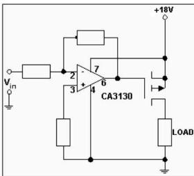
Figure 3(a). Driving Grounded Load in
