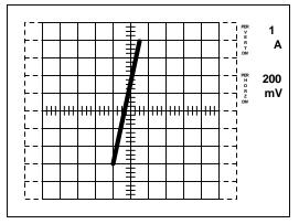
Figure 9. Source-drain voltage (diode)
