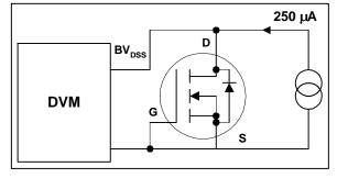
Figure 13. Test circuit for BV<sub>DSS</sub>
