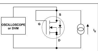
Figure 24. Test circuit MOSFET diode drop
