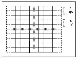
Figure 5. Gate-source leakage current at +20 V
