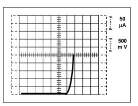
Figure 4. Gate-source threshold voltage
