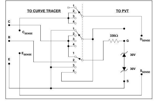
Figure 25. Test fixture for HEXFET test
