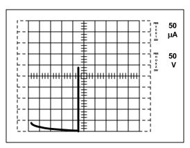
Figure 2. Drain-source breakdown voltage
