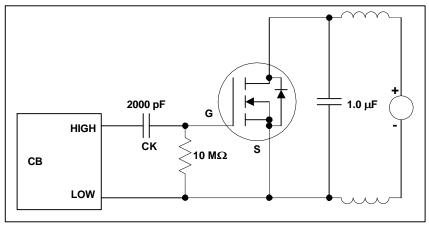
Figure 17. Test circuit for input capacitance
