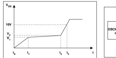
Figure 23. Gate charge waveforms
