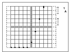
Figure 12. Transfer characteristic (I<sub>D</sub> vs V<sub>gs</sub>)
