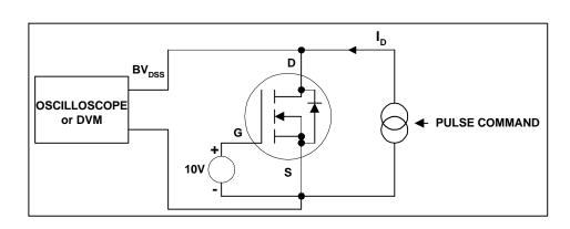
Figure 15. Test circuit for drain on-state voltage
