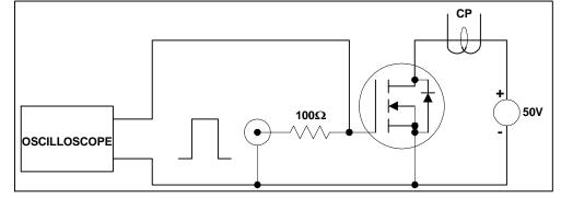
Figure 16. Test circuit for transconductance
