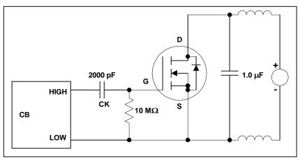
Figure 18. Test circuit for output capacitance
