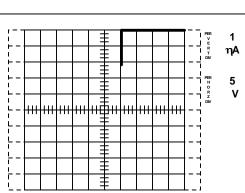
Figure 6. Gate-source leakage current at -20 V
