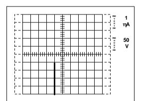
Figure 3. Drain-source leakage current
