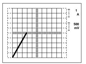
Figure 8. Drain-source resistance
