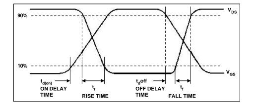
Figure 21. Switching time waveforms
