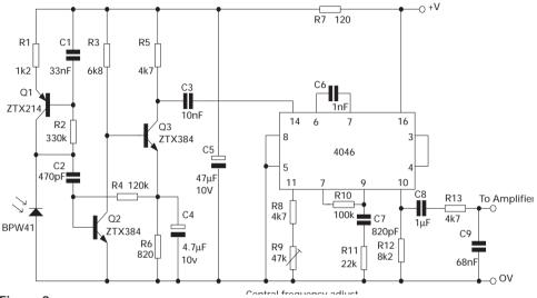
Figure 9a M.A.L. Receiver and Detector.
