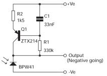
Figure 6 Active load photodiode circuit -2.
