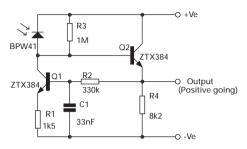
Figure 7 Active load photodiode circuit - 3.
