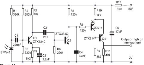
Figure 11 B.I.D. System receiver for short range duty.
