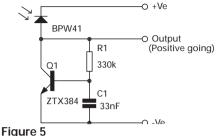
Active load photodiode circuit -1.
