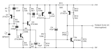
Figure 12 B.I.D. System receiver for long range duty.
