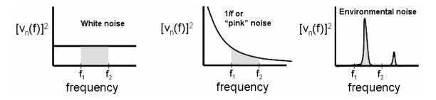
If a source that has a voltage noise spectrum given by vn(f) is measured over some range of frequencies extending from frequency f1 to frequency f2, then the mean-square noise is given by:
