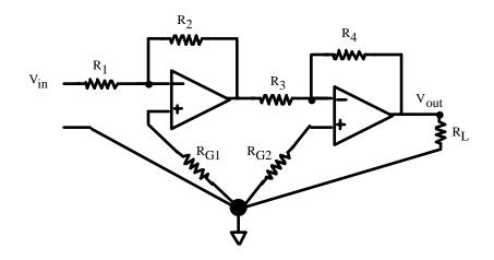
$(V_{out1} - V_{-2})/R_3 = (V_{-2} - V_{out2})/R_4$ . As before,  $V_{out1} = -V_{in}*R_2/R_1$ . Now, however,  $V_{+2} = 0$ , since it's connected directly to the "single-point" ground and because the opamp inputs draw no current (at least, for an ideal op amp). We get  $V_{out2} = R_2R_4/(R_1R_3)*V_{in}$ . The voltage measured at the output is still going to be the voltage drop across RL, which is:
