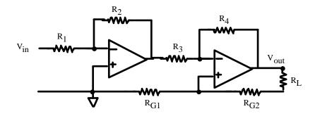
For op-amp 1, there is no problem at all: we have  $V_{out}=-(R_2/R_1)$ \*Vin. As always, we write the equations for op-amp 2 as:  $(V_{out}-V_{-2})/R_3 = (V_{-2} - V_{out}_2)/R_4$
