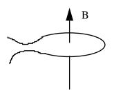
where V is the voltage induced in the loop, B is the magnetic field strength (in Tesla, where 1 Tesla =  $10^4$  Gauss) and A is the area of the loop, in square meters. (The earth's magnetic field is 0.6 Gauss, or  $6x10^{-5}$  Tesla)
