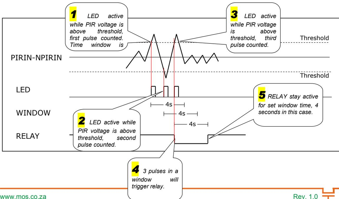
The example below shows how the alarm condition is achieved and sustained. It also shows what happens when the alarm condition does not exist any more.
