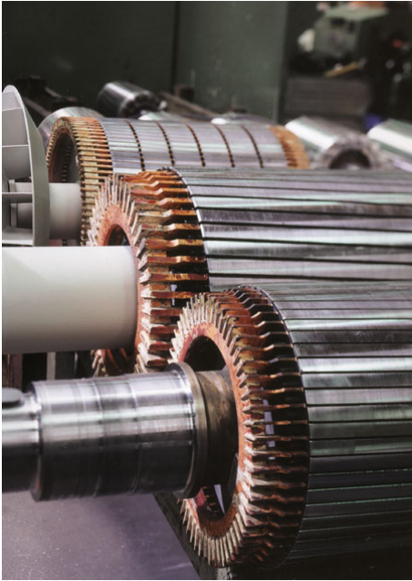
Special rotor with copper bars for efficiency increase
