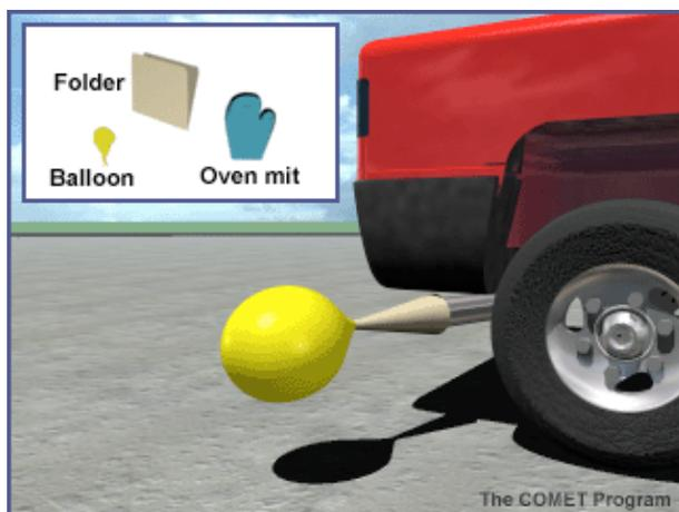
Use plenty of tape to hold the cone in shape and to make the sides of the cone fairly airtight. Note: the paper funnel will work for several fillings without burning. **DO NOT** use a plastic funnel. As the exhaust pipe heats up, the plastic may melt. You may use a metal funnel, but be **VERY** careful to avoid any skin contact with the hot metal.
