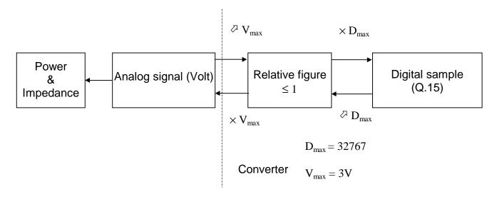
If Vmax from your converter is different, you would have to modify - by a multiply inside the routine, for example - values of transmitted samples.
