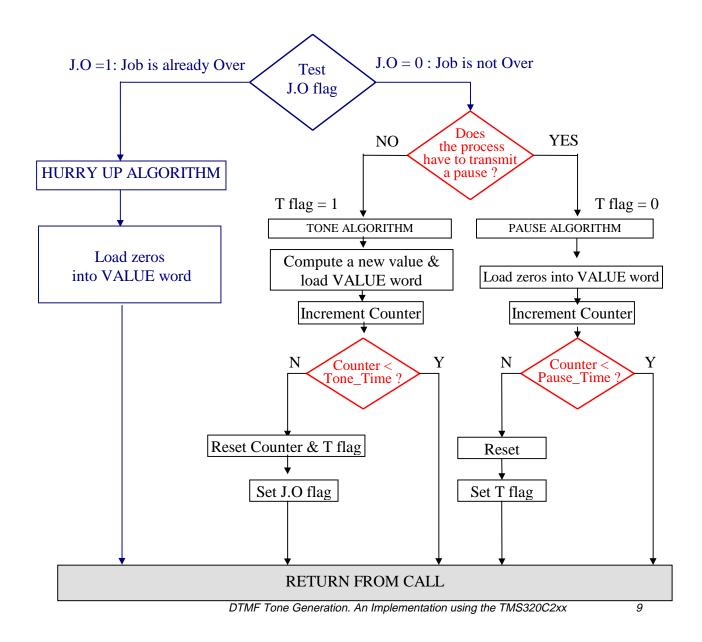
**IMPORTANT NOTICE**: The process always load VALUE with  $(y_low + y_high)(n)$ , so  $(y_low + y_high)(1)$  and  $(y_low + y_high)(2)$  won't be transmitted.
