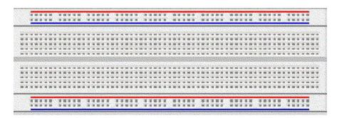
The bread board has strips of metal which run underneath the board and connect the holes on the top of the board. The metal strips are laid out as shown below. Note that the top and bottom rows of holes are connected horizontally while the remaining holes are connected vertically.
