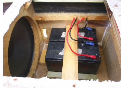
Illustration 8: Two sealed lead acid 12 volt 7AH batteries secured inside the subwoofer chamber
