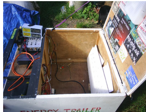
Illustration 3: Inside the body, showing forward storage space and rear electronics/audio compartment
