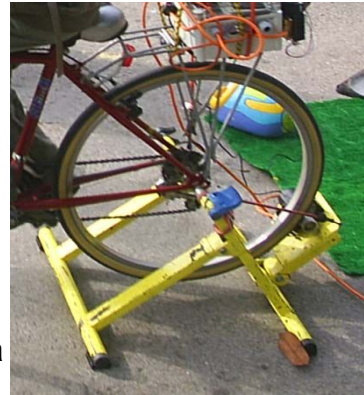
Illustration 5: Generator (car wiper motor) driven directly by back wheel
