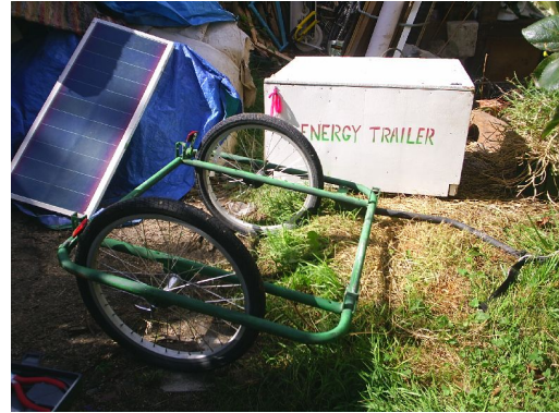
Illustration 2: Trailer chassis and body separated
