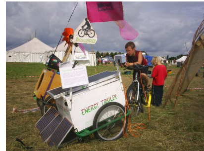
Illustration 6: Trailer with supplemental 5 watt solar panels in use
